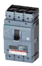
circuit breaker 3VA6 UL frame 400 breaking capacity class M 35kA @ 480 V 3-pole, line protection ETU850, LSI, In=250A overload protection Ir=100A ...250A short-circuit protection Isd=0.6..10x In, Ii=1.5..12x In N conductor protection opt. w. ext. CT; up to 160% cable connection on both sides
