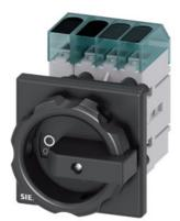
Load disconnector 3LD3, Iu 63 A Main switch 3-pole + N Rated operating capacity at AC-23 A at 400V 22.0 kW Front plate mounting Basic switch with Central hole mounting 22.5mm Toggle drive black 66x66 mm
