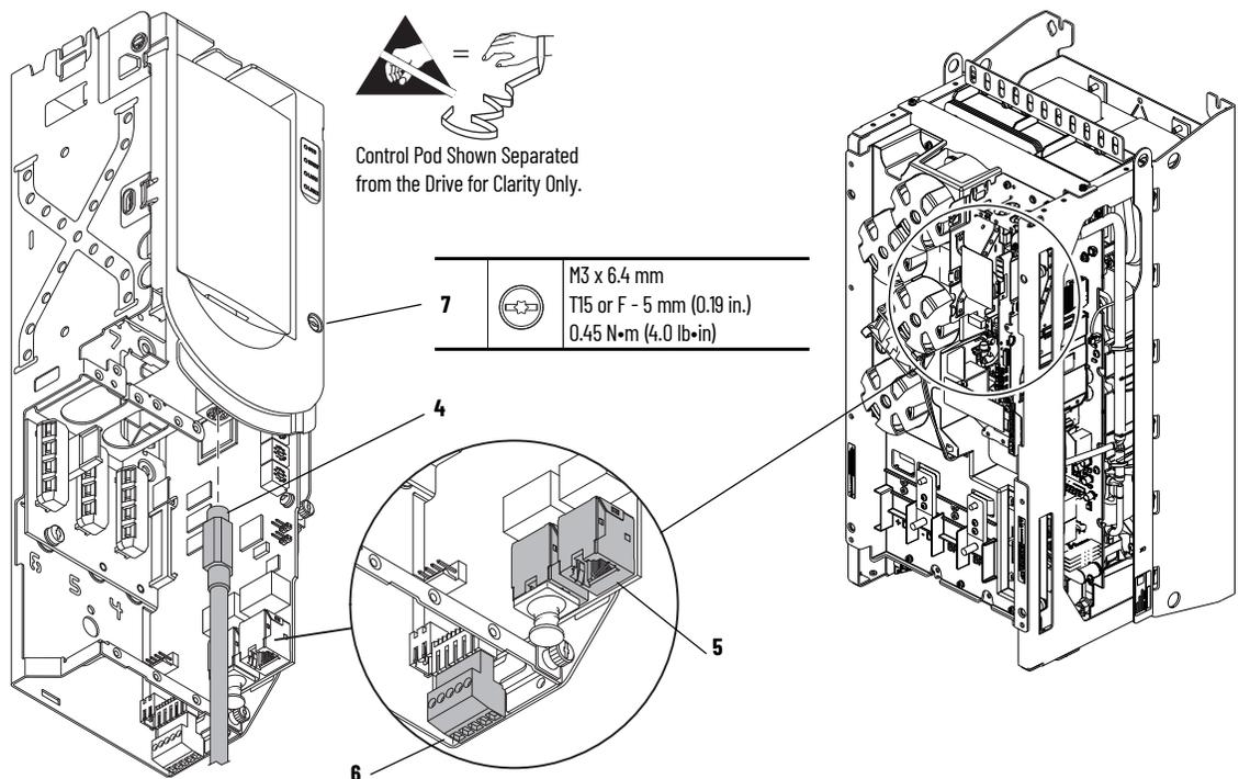
9. Disconnect the terminal block for the HIM DPI wire harness from the connector on the main control circuit board.
