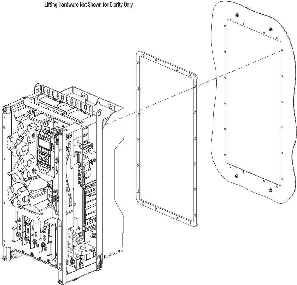
14. Remove the four M5 x 0.8 hexagonal nuts that secure the rear gasket and flange to the panel mount surface, and remove the gasket and flange. Discard the gasket.
