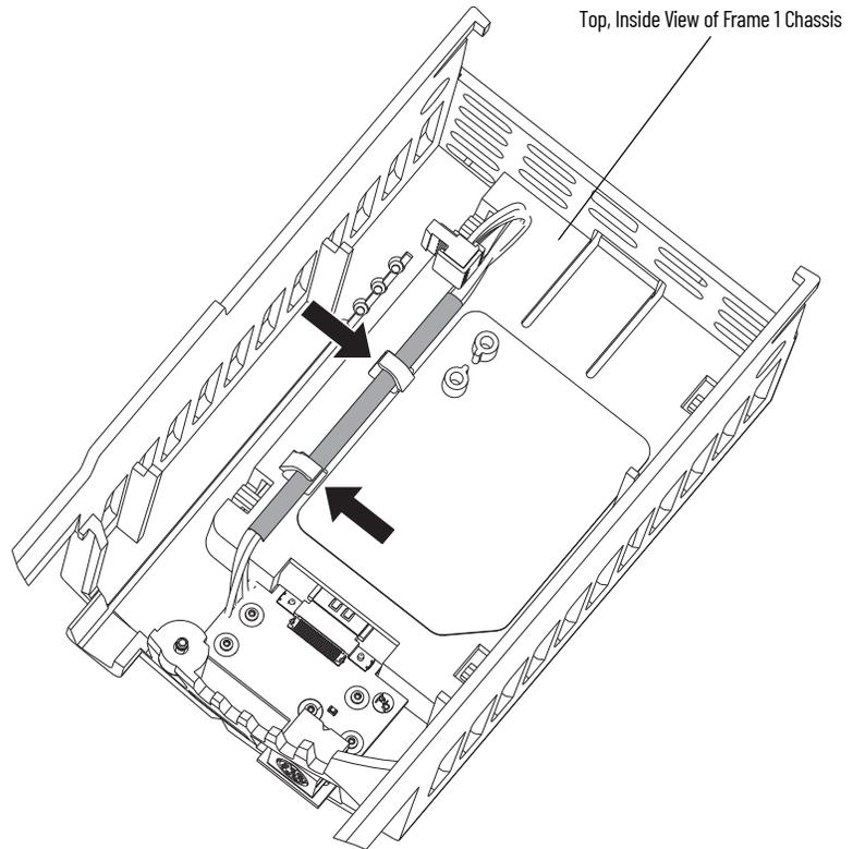
3. If a HIM and DPI cable is used, remove the protective cover from the HIM and DPI connectors on the chassis.
