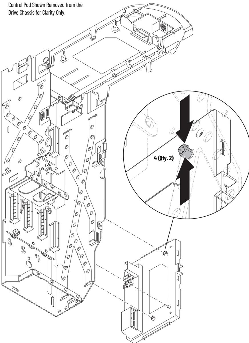
5. Remove the ribbon cable connector from the mounting tab on the inside of the control pod chassis and push the cable through the bottom of the chassis.
