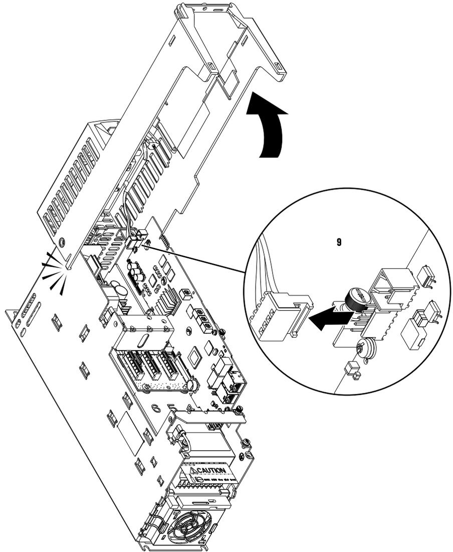
10. At the top of the plastic chassis, pull outward on the tabs and lift the chassis off the drive.
