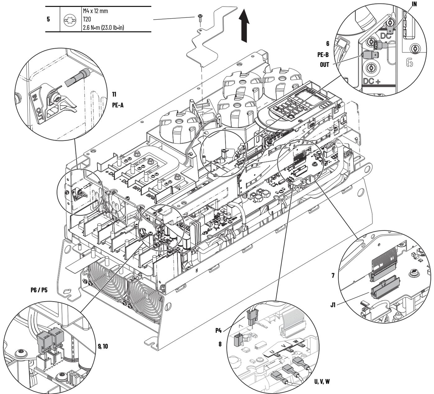
12. For drives with DC bus bars or a dynamic brake option installed, remove the applicable M6 hexagonal nuts from the bus bar terminals.
