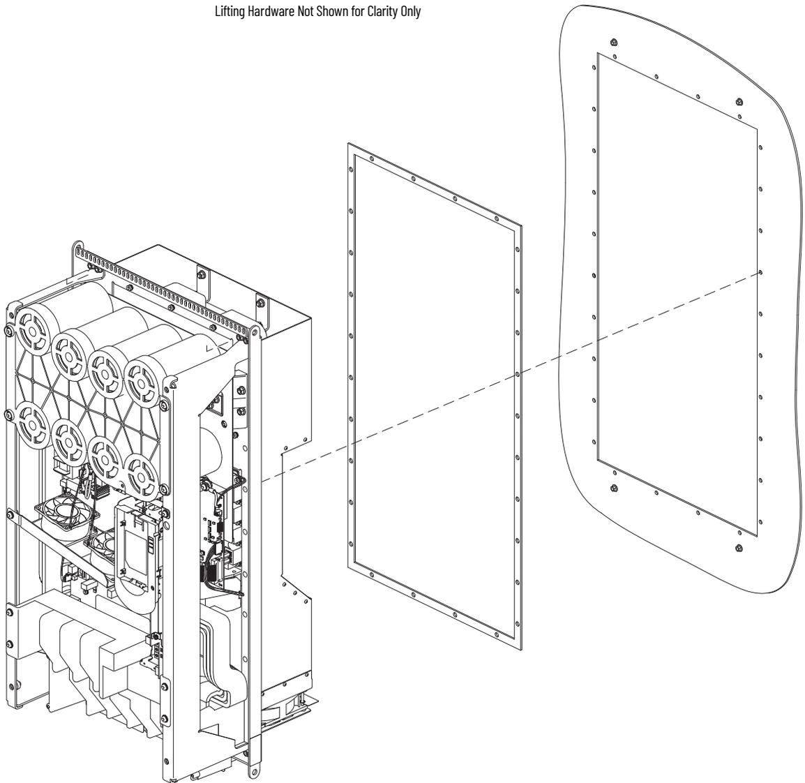
14. Remove the four M5 x 0.8 hexagonal nuts that secure the rear gasket, support brackets, and flange to the panel mount surface, and remove the gasket, brackets, and flange. Discard the gasket.
