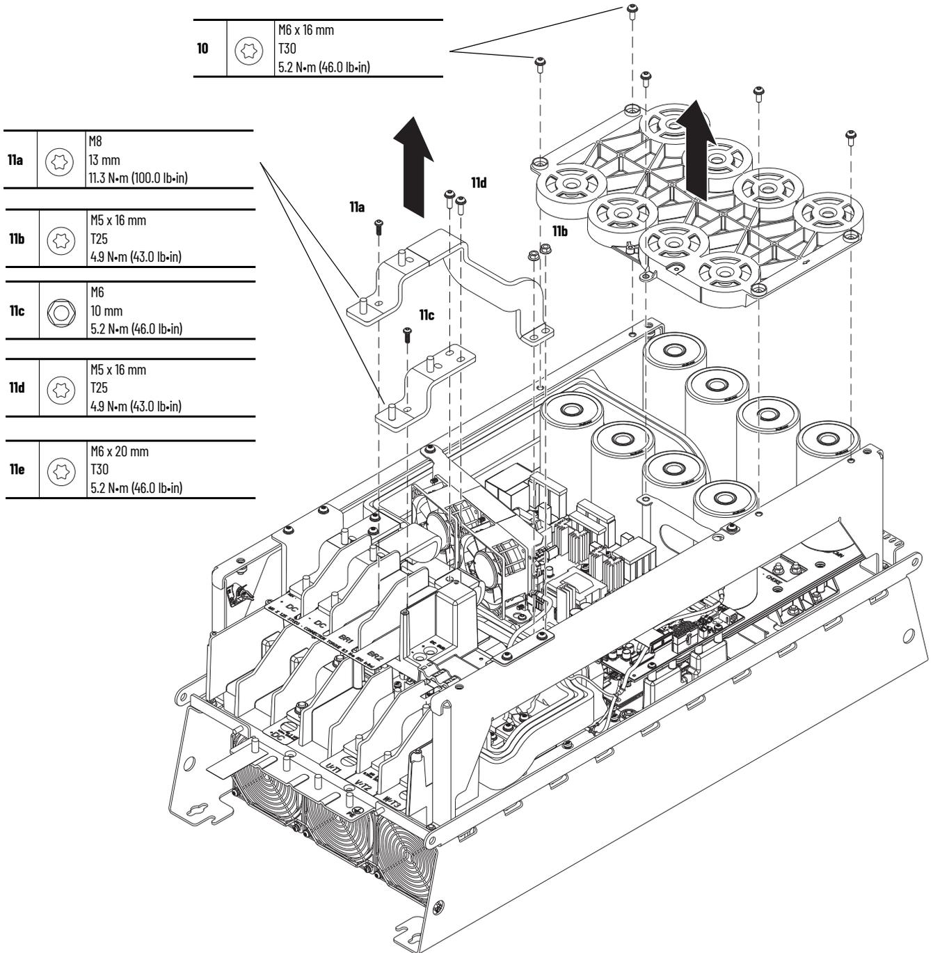
12. Loosen the two lower M5 Torx screws that secure the lower stirring fan assembly to the chassis.
