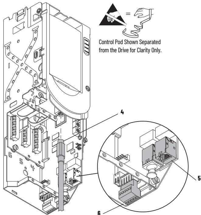
8. Loosen the screw that secures the HIM cradle to the pod chassis, and rotate the cradle up to a 90° horizontal position.
