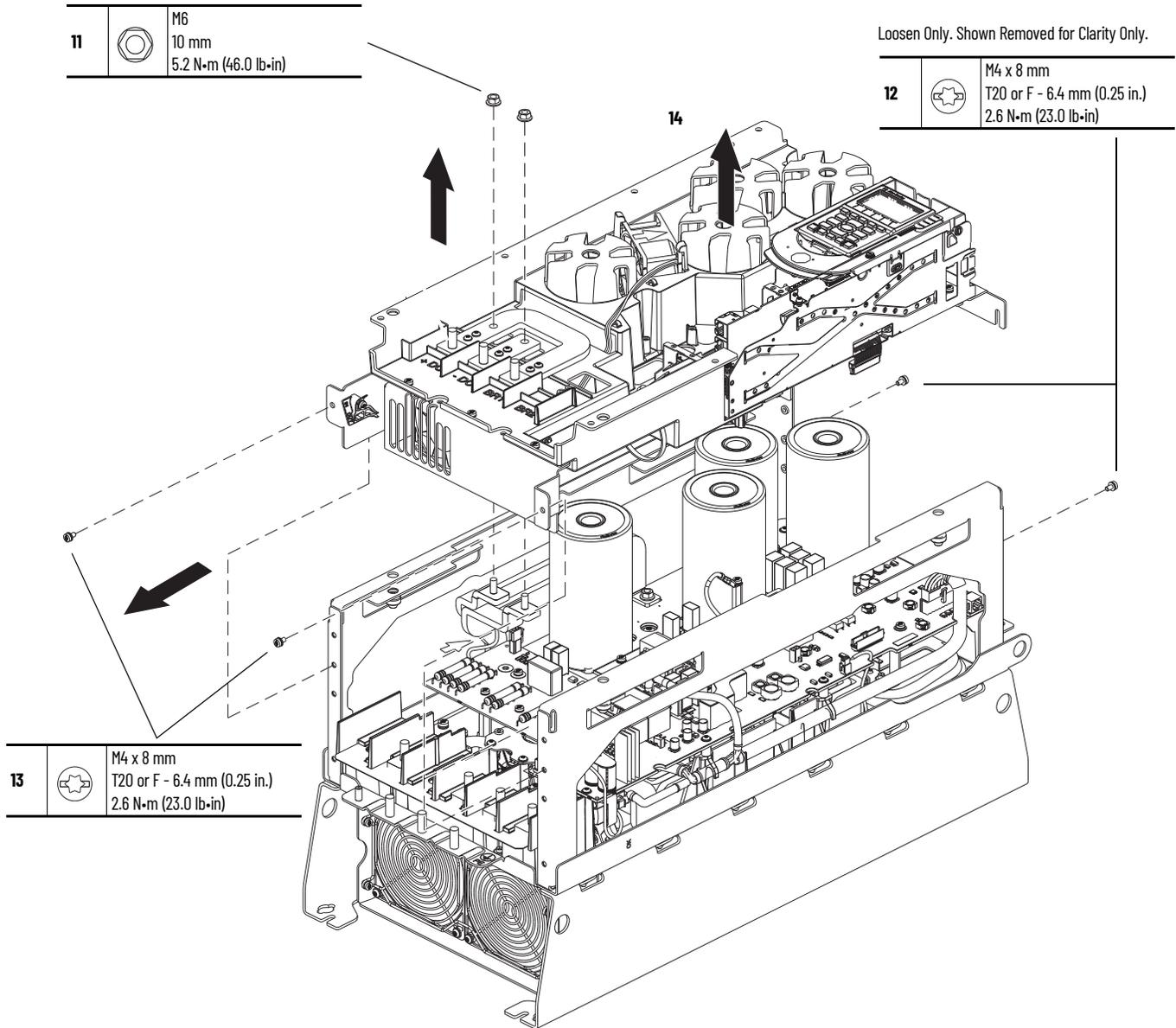
15. For DC input drives with a dynamic brake option installed, remove the M6 hexagonal nut that secures the brake bus bar to the +DC bus bar.
