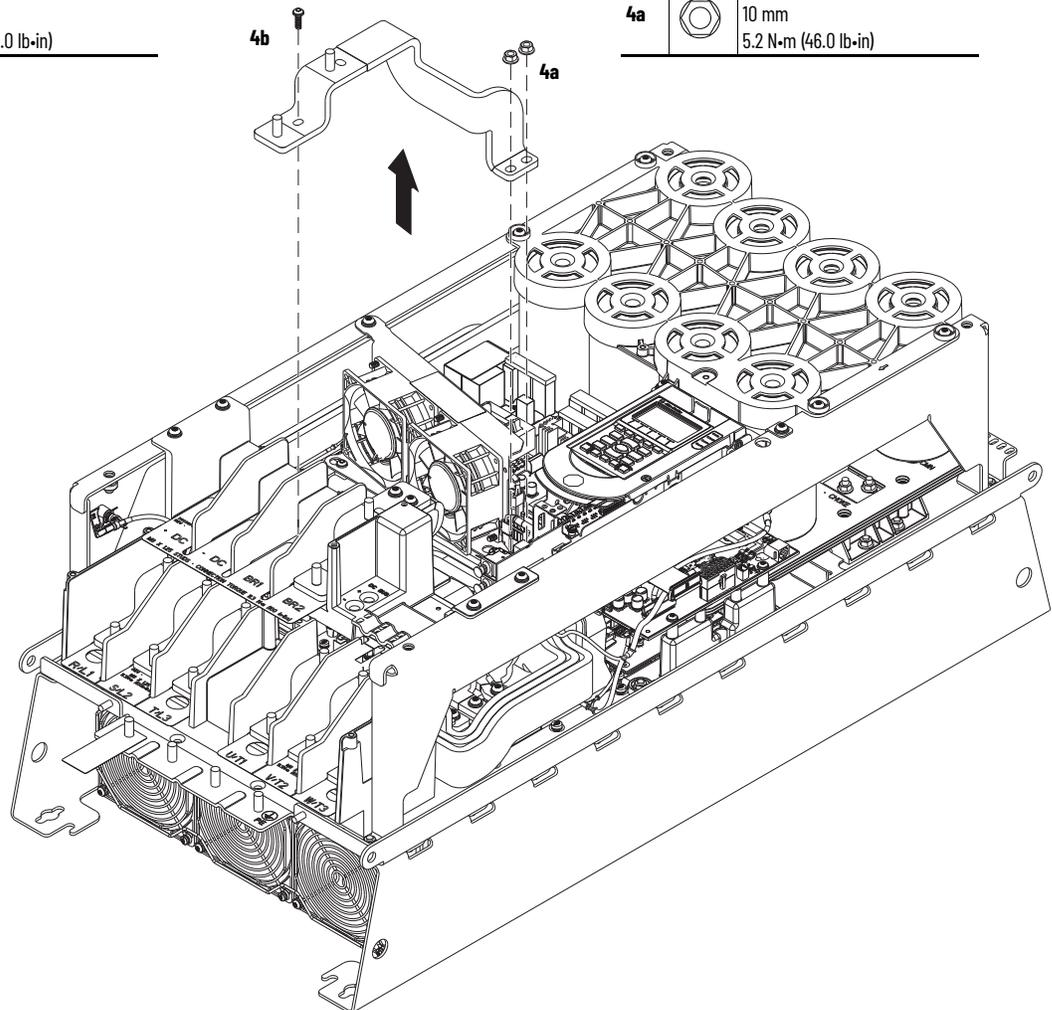
5. Loosen the two lower M5 Torx screws on the stirring fan assembly.
