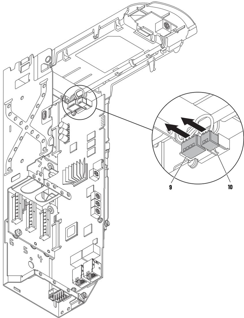
11. Record any application-specific settings on these main control board switches or jumpers (identified in this illustration):
