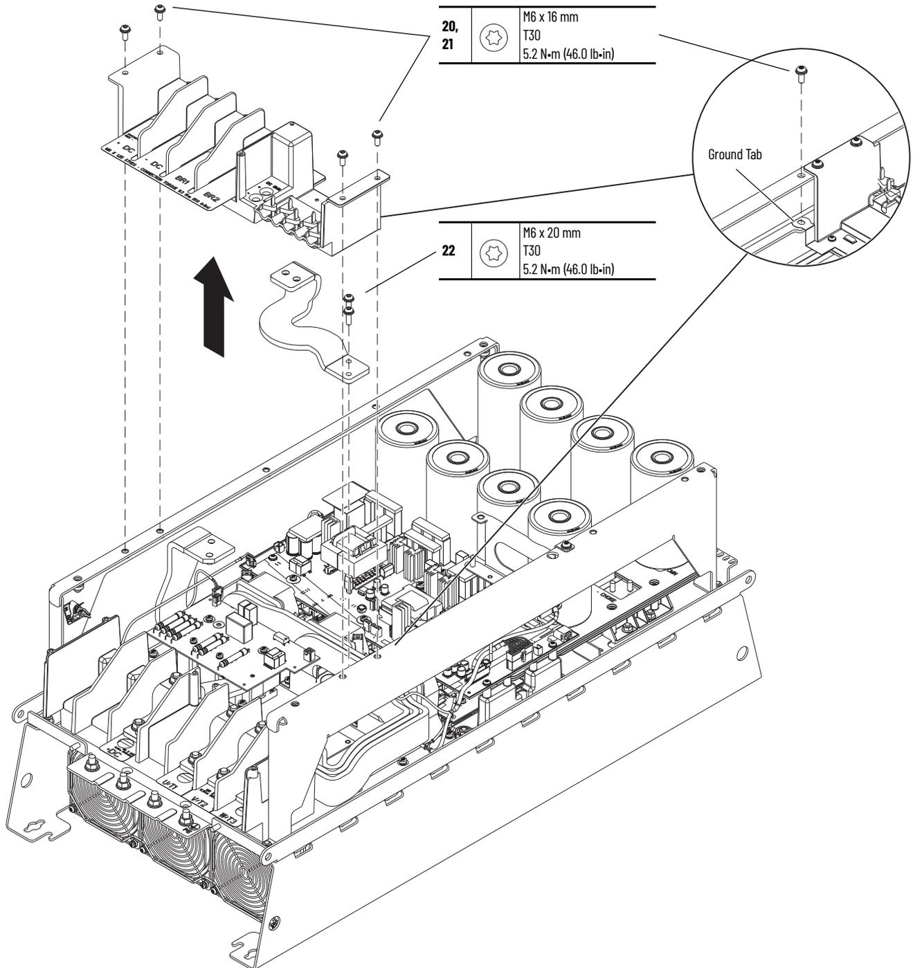
23. Remove the IGBT wire harness P11 from connector J11 on the left side of the AC precharge circuit board.
