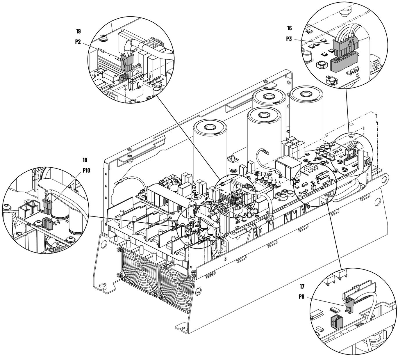
20. Remove the M4 x 8 mm slotted-Torx screw and metal tab from the M4 standoff on the power interface circuit board.
