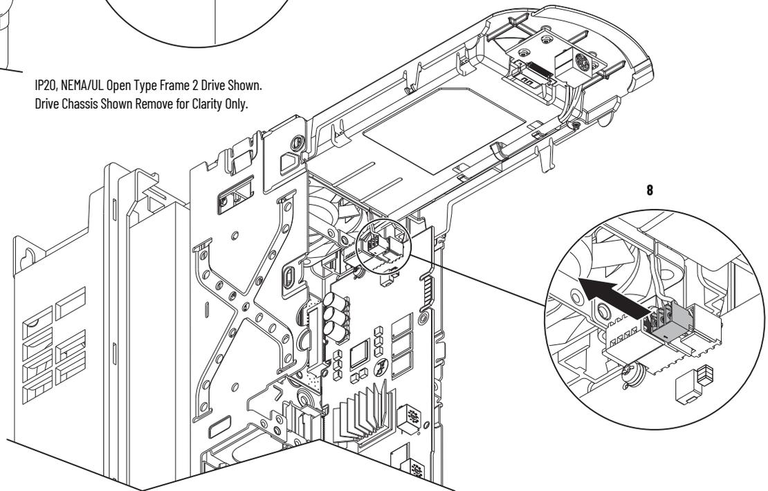
9. Press in on the two tabs on either side of the fan and remove the fan from the chassis.
