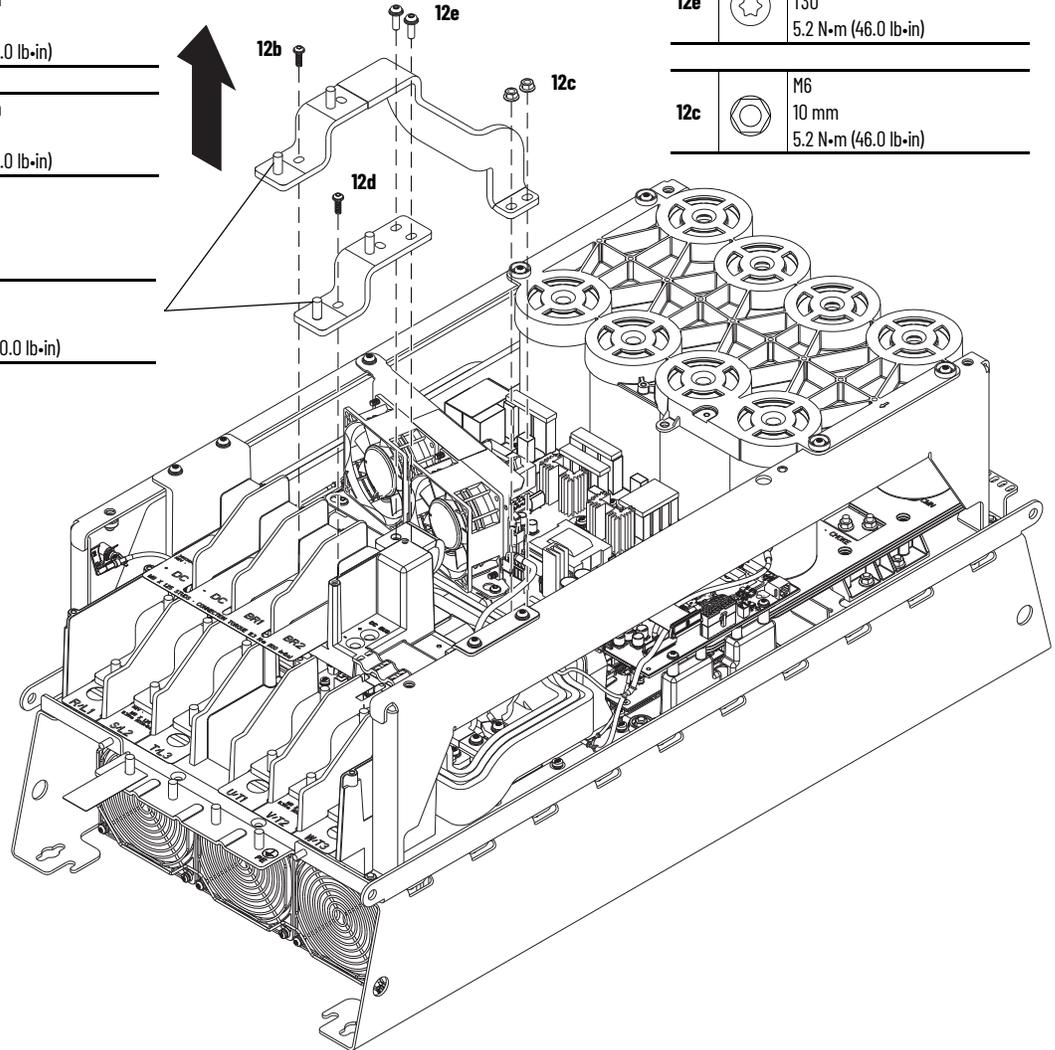
13. Loosen the two lower M5 Torx screws that secure the lower stirring fan assembly to the chassis.
