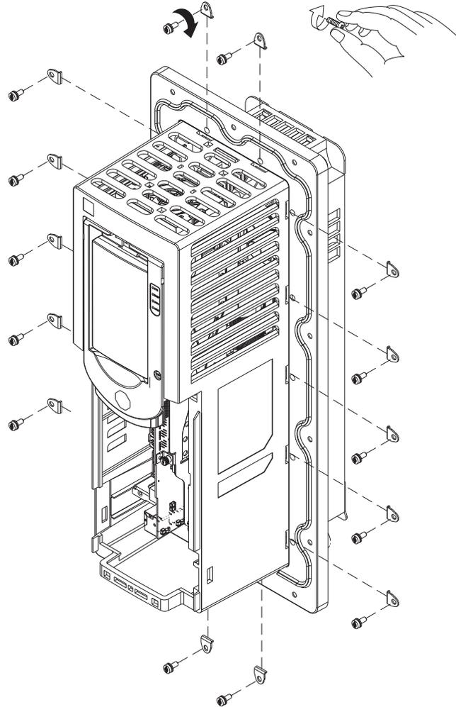
3. To secure the drive to the flange, apply final torque by using the sequence that is shown.
