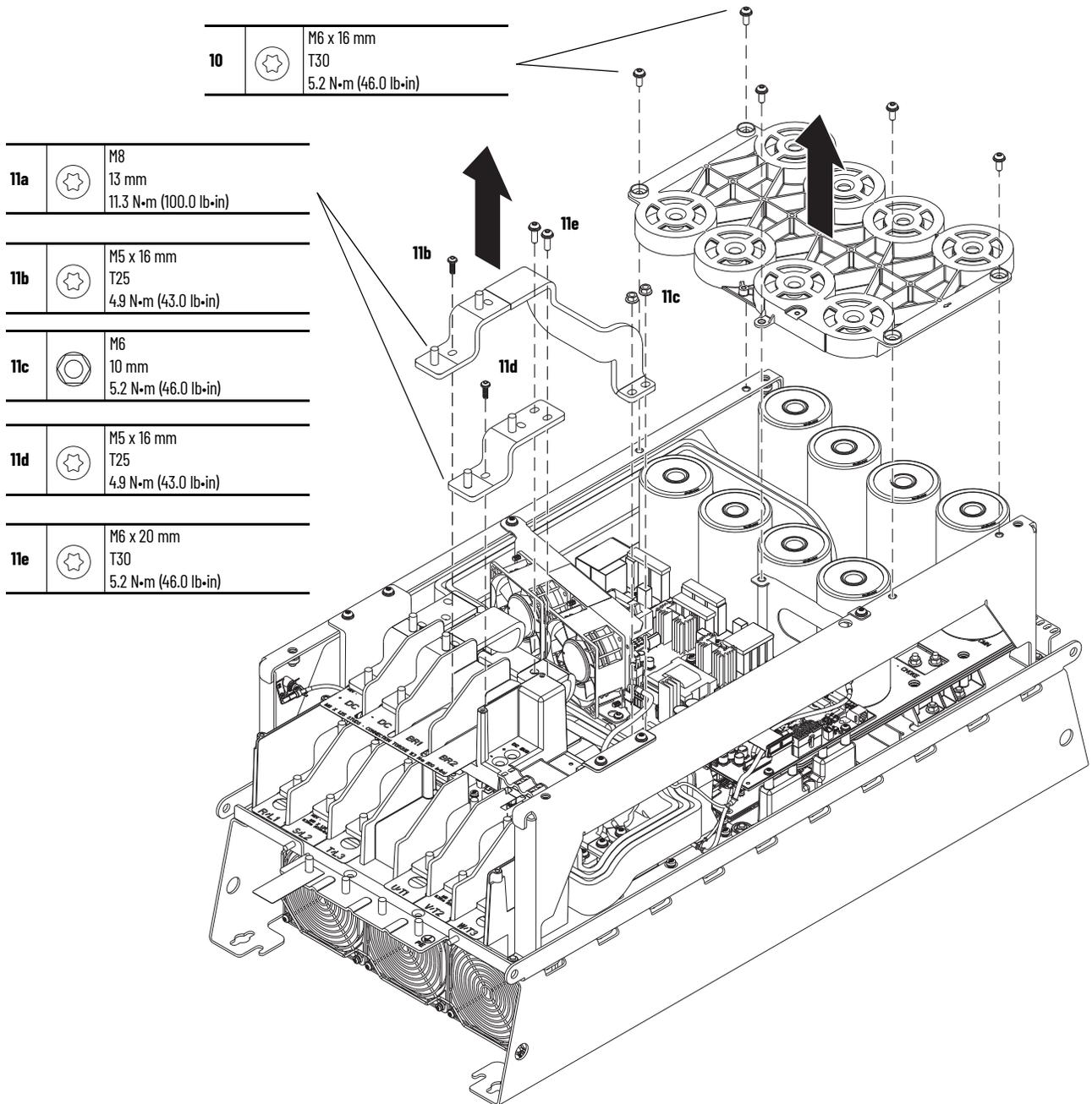
12. If the DC bus bars are installed, complete steps a..d to remove the stirring fan assembly.
