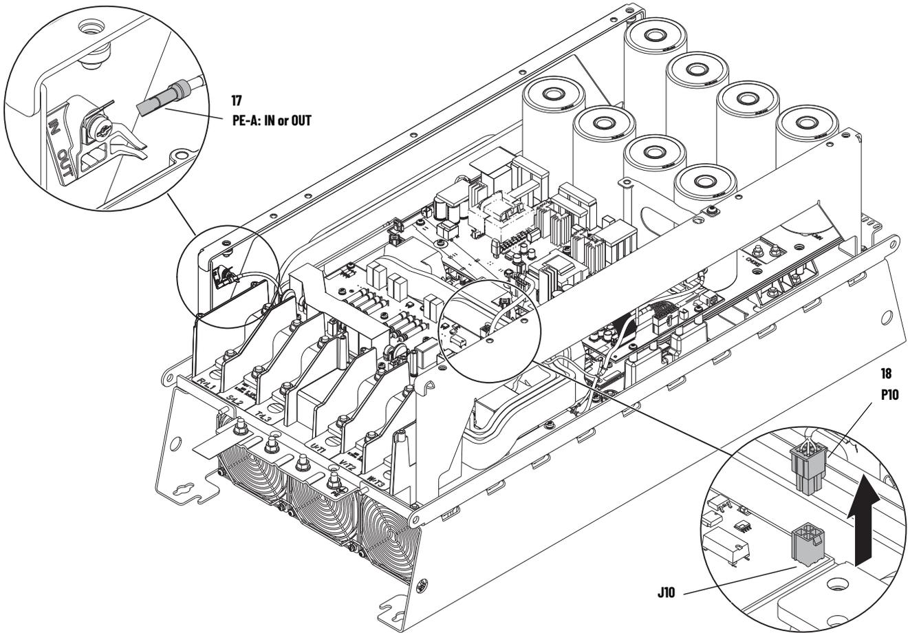
19. Remove the nine M4 x 8 mm slotted-Torx screws that secure the board to the standoffs.
