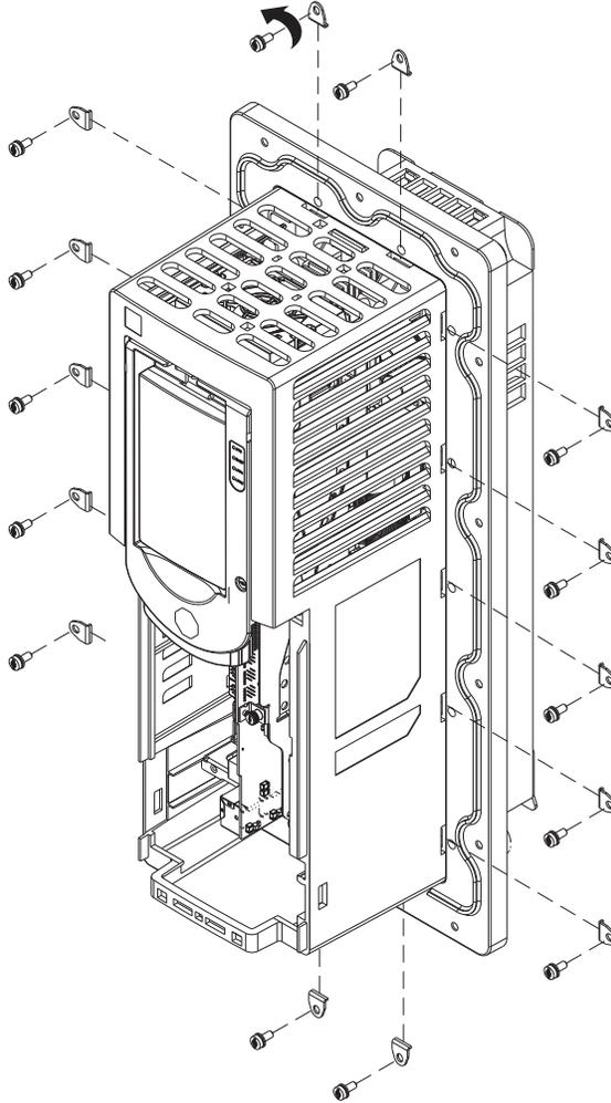
11. Remove the gasket from the flange and discard.
