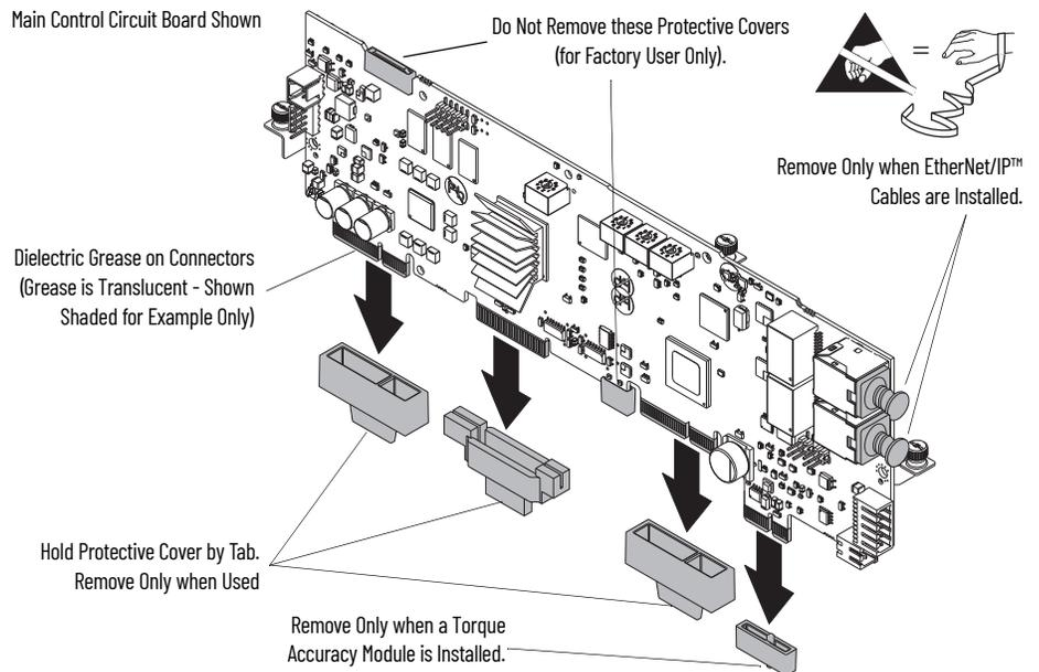
**IMPORTANT** If before installation, grease is removed from an edge connector or is contaminated, do not install the circuit board. See [Apply Dielectric Grease to an Edge Connector on page 16](#) for instructions on how to clean and grease an edge connector.
