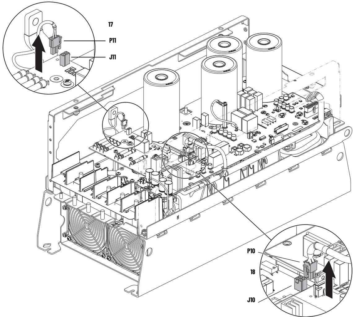
19. Remove the four M4 x 8 mm slotted -Torx screws that secure the DC precharge circuit board to the standoffs and remove the board.
