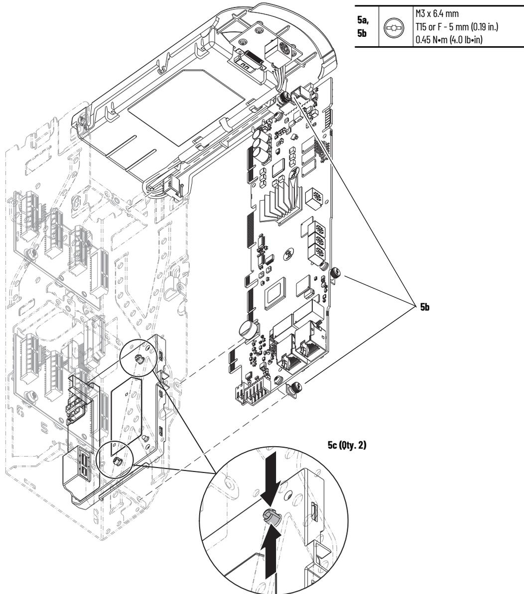
6. Disconnect the ribbon cable from connector J1 on the power interface circuit board below the control pod.
