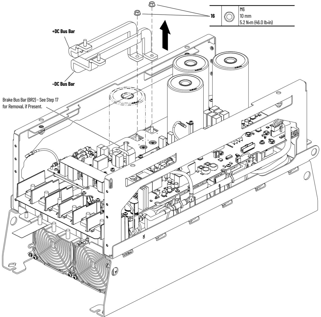
17. If a brake bus bar is installed, complete steps a...i to remove the power interface circuit board.
