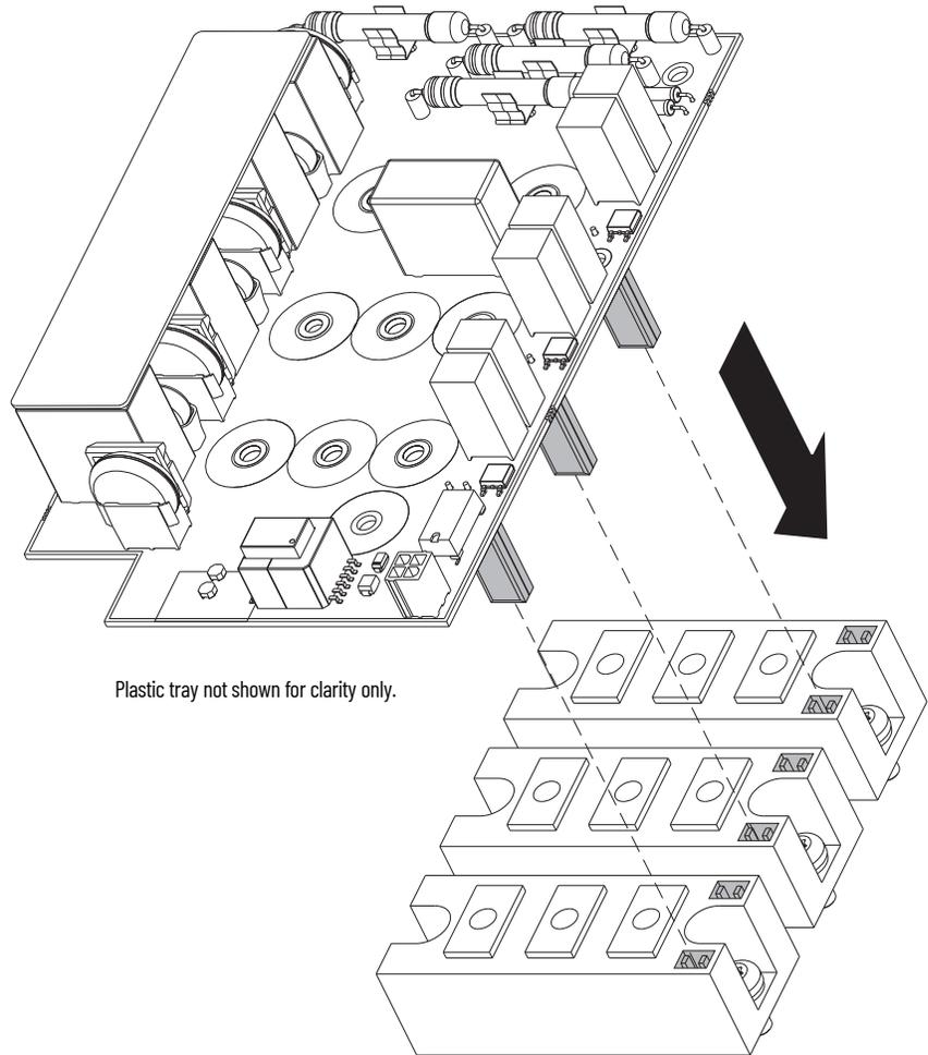
4. Install the AC precharge circuit board in the reverse order of removal.
