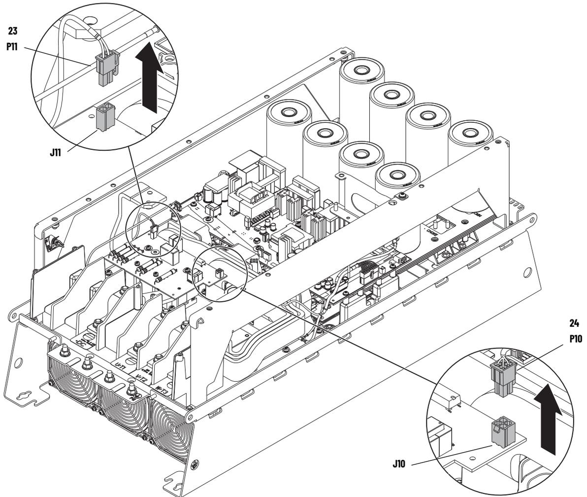
25. Remove the four M4 x 8 mm slotted-Torx screws that secure the DC precharge circuit board to the standoffs and remove the board from the drive.
