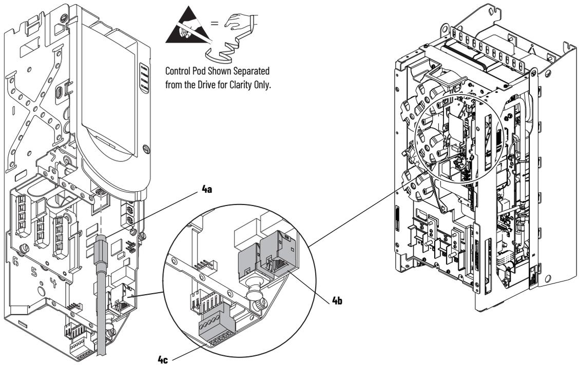
5. Remove the M4 x 12 mm Torx screw that secures the PE-B jumper cover to the capacitor cover and remove the jumper cover.
