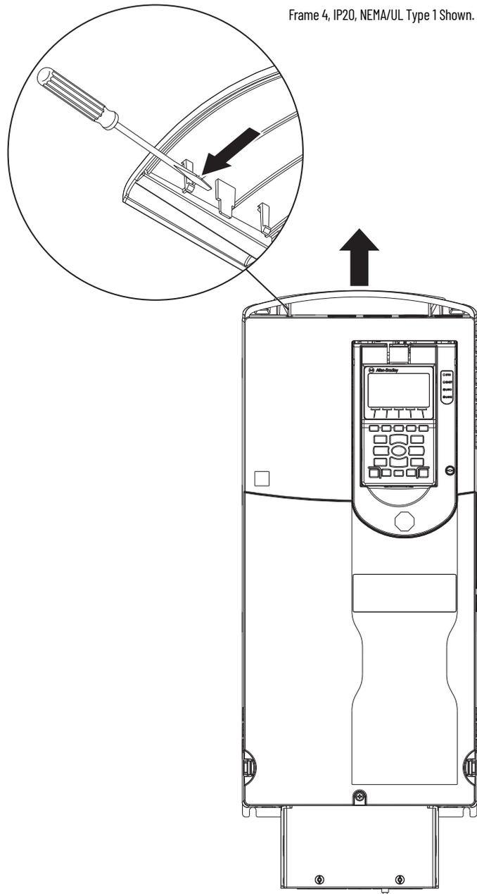
4. Remove the power terminal cover. See [Remove the Power Terminal Cover, Frames 1...5 on page 31](#).
