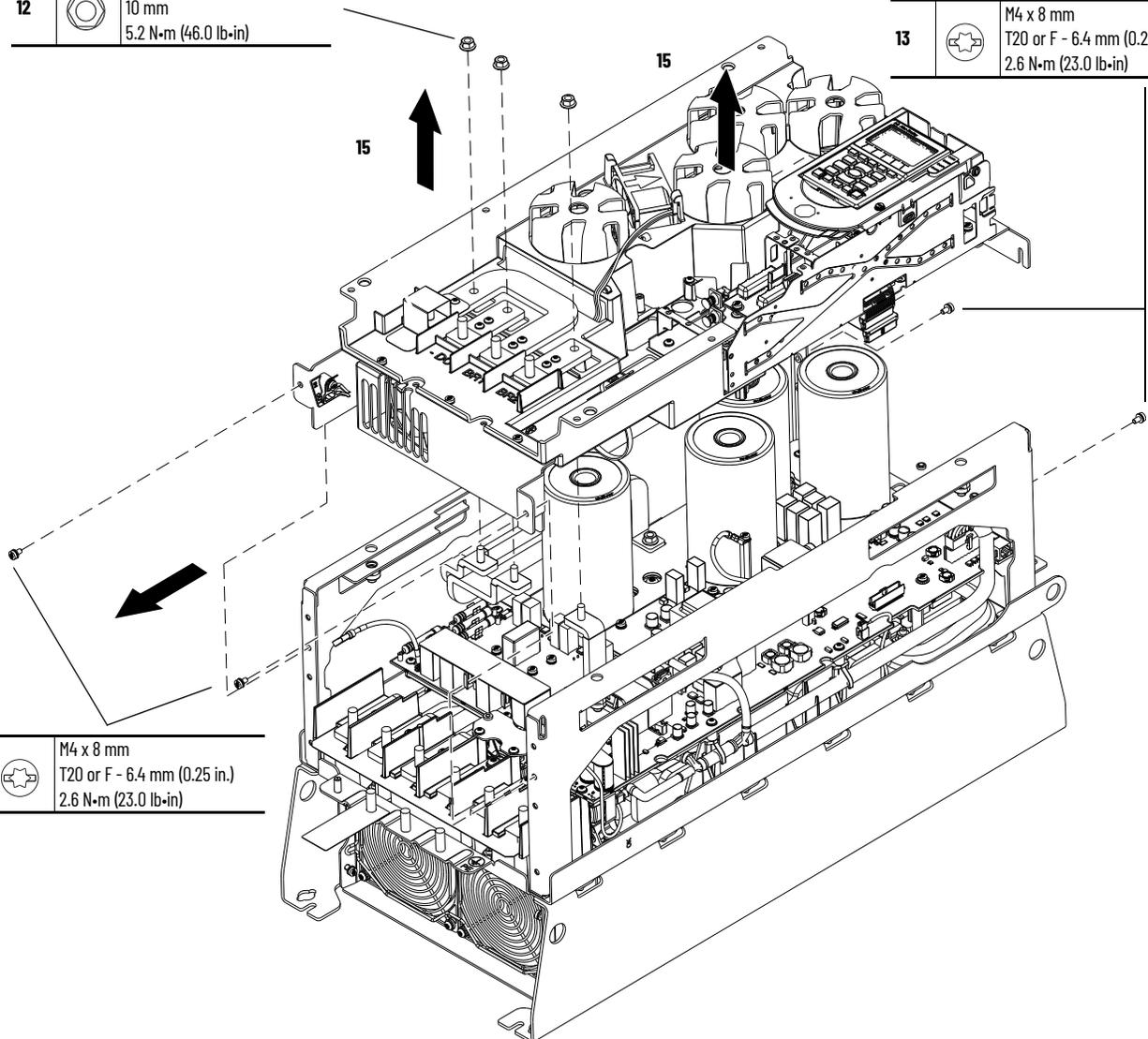
16. If the DC bus bars are installed, remove the two M6 hexagonal nuts that secure the DC bus bars to the laminated bus.
