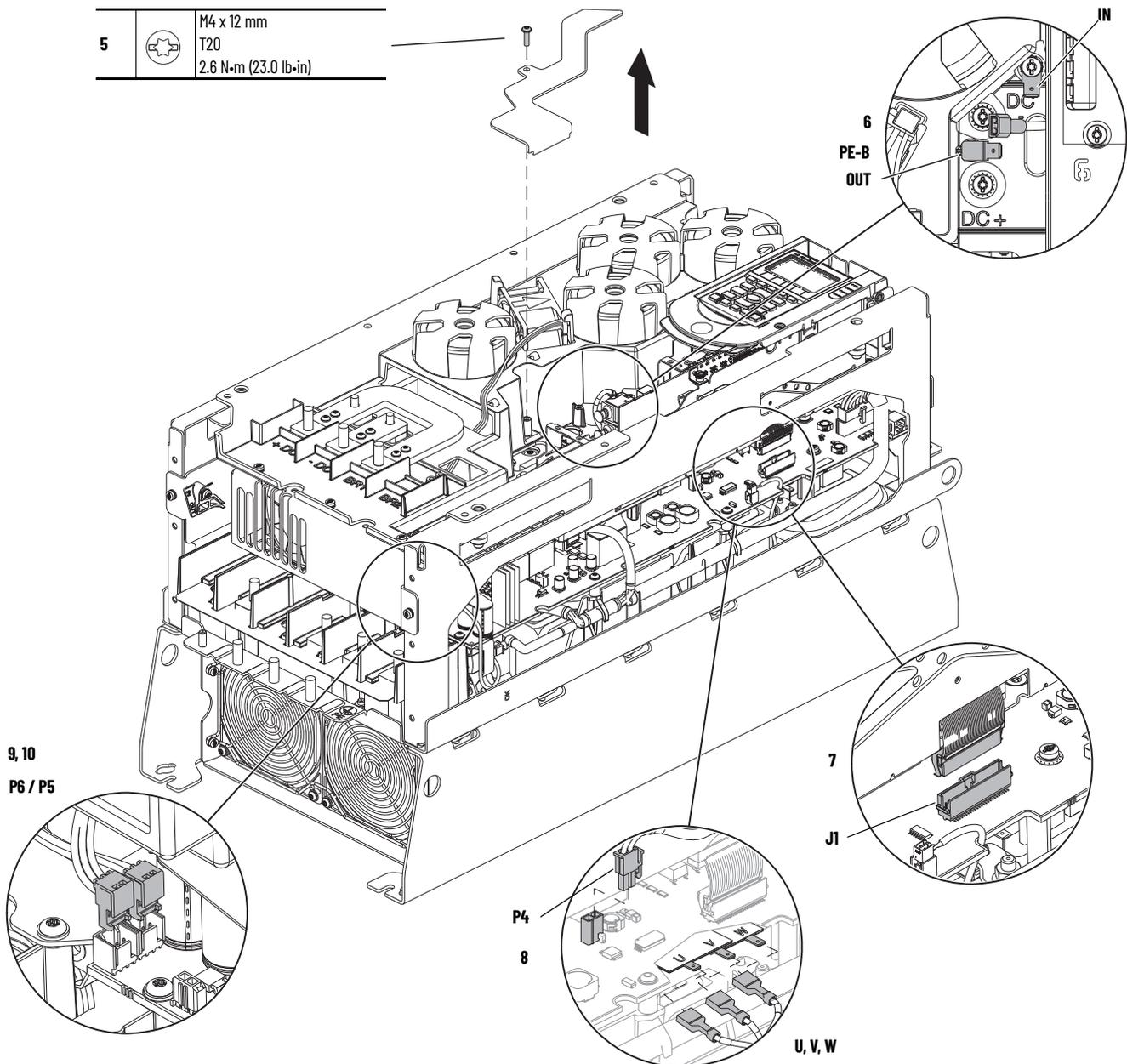
11. Remove the M6 hexagonal nuts from the DC bus bar terminals.
