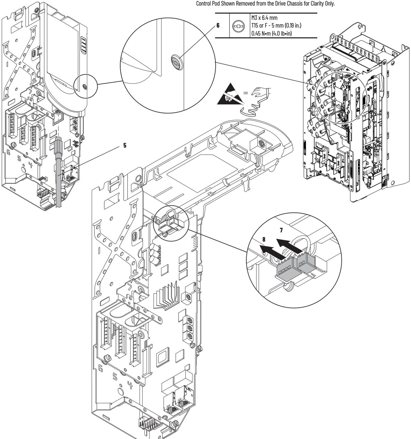
9. Press in on the tabs at the top of the HIM cradle where it connects to the control pod chassis to release the cradle from the chassis.
