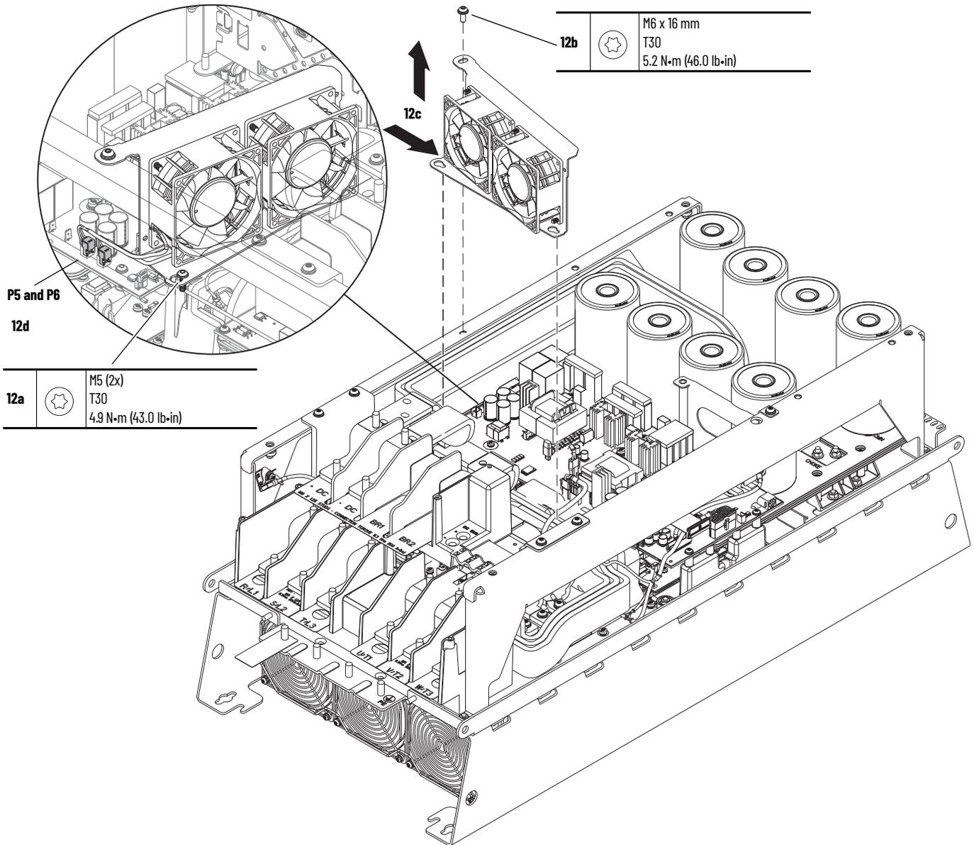
13. If the DC bus bars are installed, complete steps a and b.
