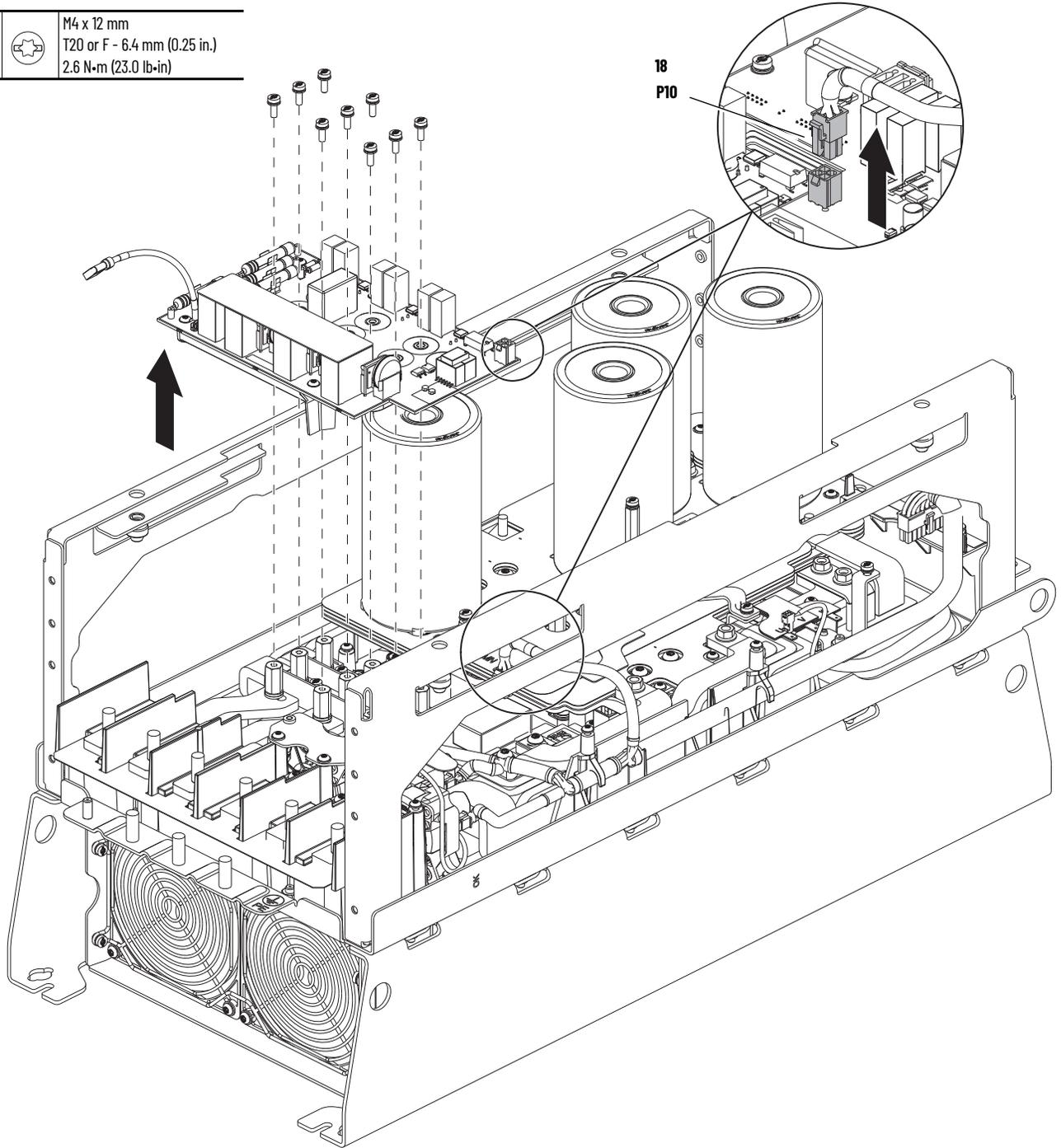
20. Remove the circuit board stiffener from the capacitors on the board.
