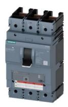
circuit breaker 3VA6 UL frame 600 max short-circuit curr. rating 100kA @ 480V w/o contactor 3-pole,motor starter protection ETU310M, I, In=400A without overload protection short circuit protection Ii=3...13 x In Al-lug, line side
