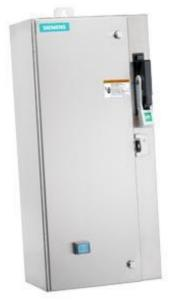
Non-reversing motor starter Size 0 Three phase full voltage Solidstate overload relay OLRelay amp range 0.75-3.4A 24VAC 50-60HZ coil Combination type 30Amp fusible disconnect 30 Amp /600V fuse clip Encl NEMA type 4X 316 S-steel Water/dust tight non-corrosive Standard width enclosure
