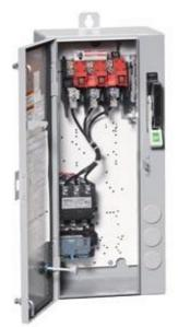
Non-reversing motor starter, Size 2, Three phase full voltage, Solidstate overload relay, OLRelay amp range 13-52a, 190 220/220 240V 50/60HZ coil, Combination type, 60Amp non-fused disconnect Enclosure NEMA type 4/12, Water/dust tight for outdoors, Standard width enclosure
