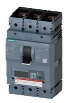
circuit breaker 3VA6 UL frame 600 breaking capacity class L 150kA @ 480 V 3-pole, line protection ETU550, LSI, In=600A overload protection Ir=240A ...600A short-circuit protection Isd=0.6..9x In, Ii=1.5..9x In N conductor protection opt. w. ext. CT; up to 160% nut keeper kit on both sides
