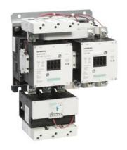
Reversing motor starter Size 5 Three phase full voltage Solid-state overload relay OLRelay amp range 55-250A 575-600V 50-60HZ/DC coil Non-combination type Enclosure type (open)
