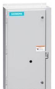
Non-reversing contactor, Size 3 1/2, Three phase full voltage, Contactor amp rating 115A, 3 wire (NO aux included), 24VAC 50-60Hz coil, Non-combination type, Enclosure NEMA type 12, Dust/drip proof for indoors, Extra-wide enclosure
