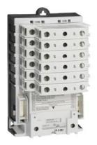
Electrically held lighting contactor, (convertible to mech. held), Amp rating 30A (tungsten 20A), 0 N.C. / 9 N.O. poles, 347V 60Hz coil, Non-combination type, Enclosure NEMA type (open), No enclosure
