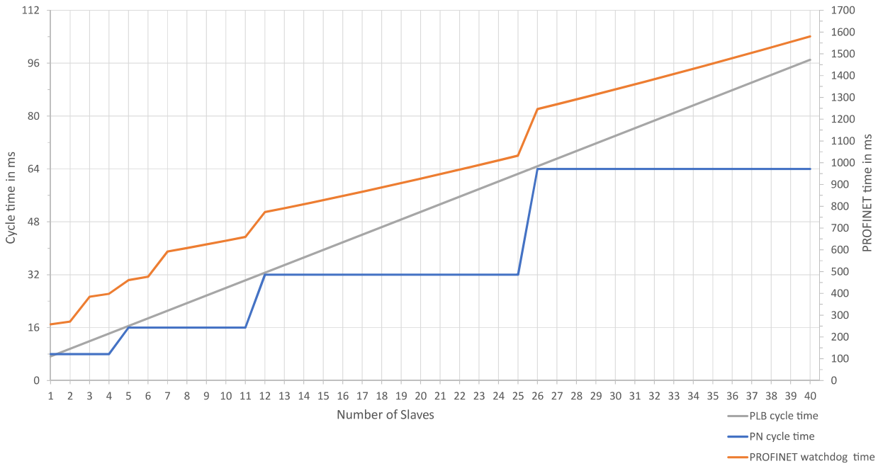
Figure 5-4 Graphic for determining the PROFINET times
