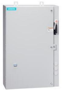
Non-reversing motor starter Size 3 Three phase full voltage Solidstate overload relay OLRelay amp range 25-100A 220-240/440-480VAC 60HZ coil Combination type 100A fusible disconnect 100A/600V fuse clip Encl NEMA type 4X 304 S-steel Water/dust tight non-corrosive Standard width enclosure
