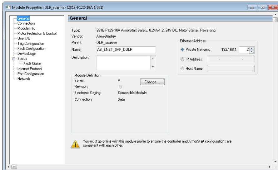
This tab lets you name your module, which must be descriptive and representative of the module. You must also input the IP address of the module so that communication can be established. The IP Address must be the one defined when the BootP/DHCP Server, the Rotary Network Address Switches, or the ArmorStart internal web server. is used.
