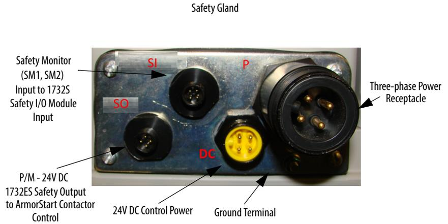
Factory-installed ArmorConnect gland plate and terminal connections
