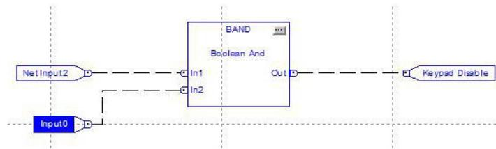
**Note:** If you are already pressing the “HAND” button, the program does not disable the keypad; if the inputs are on after the “HAND” mode is actuated.
