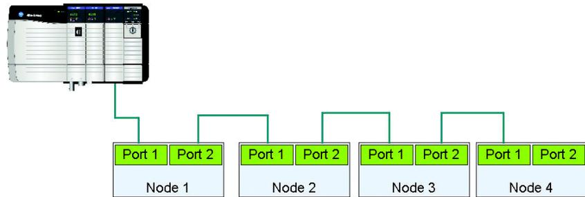
In this topology, a communication issue in the media or device helps stop nodes downstream from communicating.
