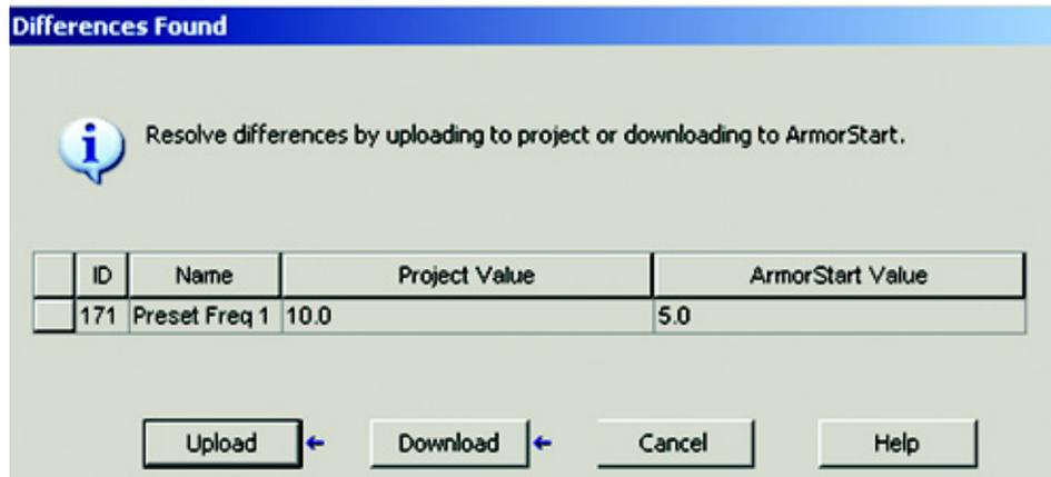
Figure 100 is an example of the DeviceLogix correlation when a difference occurs between the project and the device.
