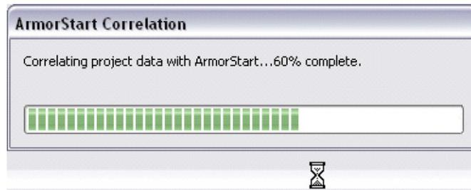
This window indicates that the AOP is comparing the parameter data entered offline vs. the parameter data that is stored in the ArmorStart device. If any discrepancies are found between the parameters in the AOP and the parameters in the ArmorStart device, a window pops up, as shown. The window prompts you to decide which parameters to keep.
