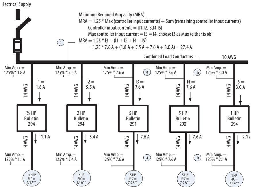
**1. Requirement One: Controller Ratings** — The motor controllers and overload relays must be listed for group installation with specified maximum branch-circuit protection.
