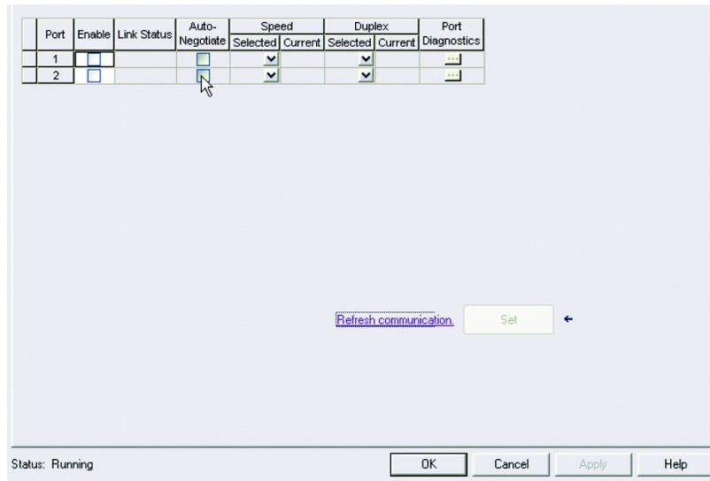
This tab is used to enable or disable a physical port in the module. The ports are normally in Auto Negotiate mode, which in general, is the recommended setting. Otherwise, you have to physically set the Speed or Duplex selection in this tab. It is important to note that although there are two physical ports, they act as one. Therefore, when you press either of the Port Diagnostic buttons, information that comes from both of the physical ports is displayed.
