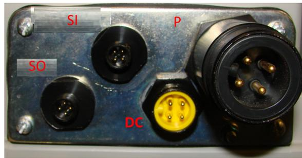
**Figure 8 - Safety Power Block Input and Output Configuration**
