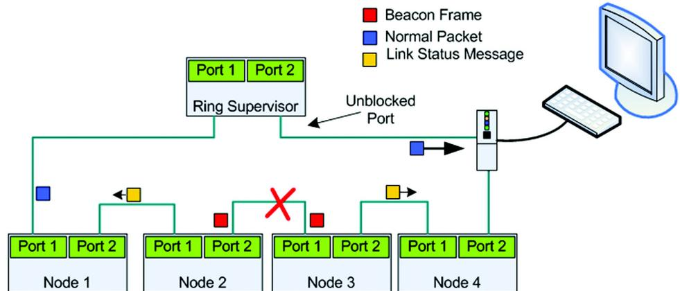
When the physical layer fault is corrected, the supervisor will “hear” the beacon frame again on both ports. Once the beacon frame is detected, the ring supervisor re-establishes and configures the ring topology. All neighboring nodes detect this update and reconfigure themselves back to ring. A DLR network is a single-fault tolerant network that is intended for the interconnection of automation devices.
