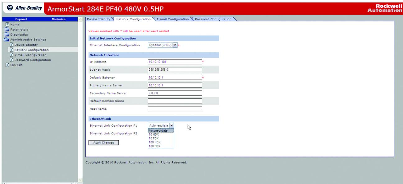
From this screen, you can change the Ethernet Configuration. In the example that is shown, the default IP address was changed from 192.168.1.1 to 10.10.10.101. To access the web page after a power cycle, the new address must be used.
