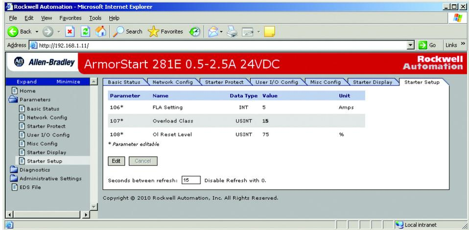
In Figure 59, the Starter set-up parameters are viewed. You can view all parameters from this screen. To modify a parameter, click the “Edit” button.
