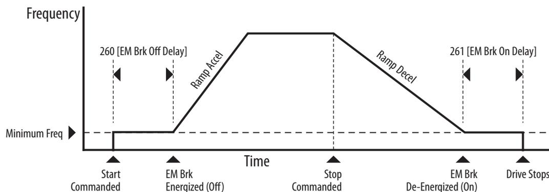
4. See the consume assembly next. The Drive Input that was configured in step #1, is used to control the mechanical brake.
