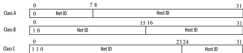
You can distinguish the class of the IP address from the first integer in its dotted-decimal IP address as follows:
