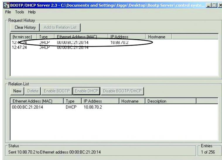
When the address displays in the IP address column in the Request History section, it signifies that the IP address assignment has been made.
