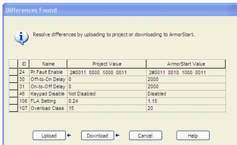
If you want to keep the parameters in the AOP, select Download. If you want to keep the parameters in the ArmorStart device, select Upload. Otherwise, select Cancel. When you click Cancel, you are locked out of viewing the values. If you are connected to a new ArmorStart device and just created the ArmorStart object and have not made changes in the parameters, the ArmorStart correlation must not find any discrepancy.
