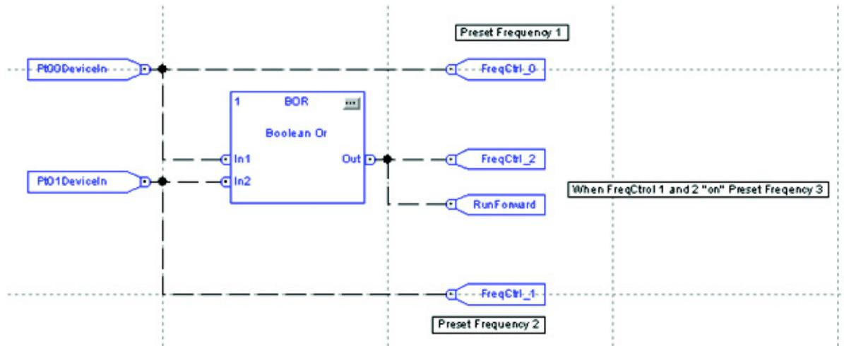
Once you exit the DeviceLogix editor, verify that the logic is “Enabled” otherwise the preset frequency control does not operate. See Figure 98.
