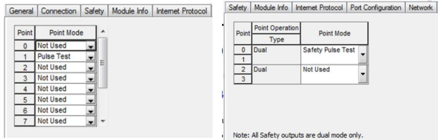
Configure the input that is connected to the I/O Input cable assembly as follows:
