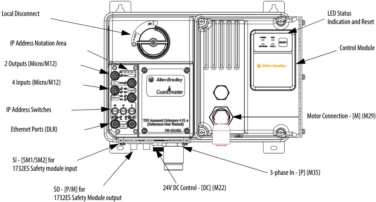
Figure 14 - Bulletin 284E ArmorStart ST - Safety Starter
