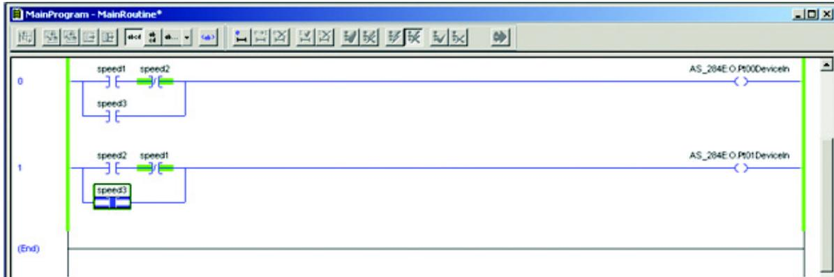
Download the finished program file to the PLC. In order for the parameters and DeviceLogix program to update in the device, verify that the PLC is in program mode, and open the AOP for the Bulletin 284E controller.
