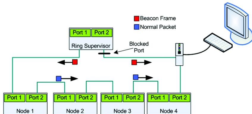
As shown in [Figure 44](#), when a physical layer failure is detected the adjacent nodes to the fault generate a link status message that the ring supervisor acknowledges. The ring supervisor unblocks the port to allow communication. The neighboring nodes to the fault identify the fault and reconfigure themselves to support a linear topology. Now, both the ring supervisor and nodes are configured to support a linear topology.
