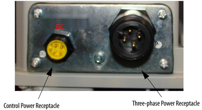
Factory-installed ArmorConnect gland plate and terminal connections
