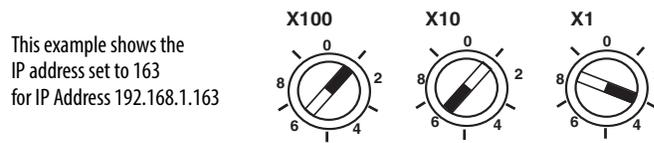
Valid IP address switch settings range from 002 to 254. When the switches are set to a valid number, then the IP address of the adapter is 192.168.1.xxx (where xxx represents the number set on the switches; see [Figure 48](#)). The subnet mask of the adapter is 255.255.255.0 and the gateway address is set to 192.168.1.1. A power cycle is required for any new IP address to take effect.
