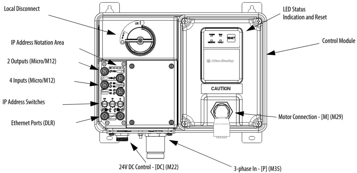
Figure 12 - Bulletin 284E ArmorStart ST DOLR Starter
