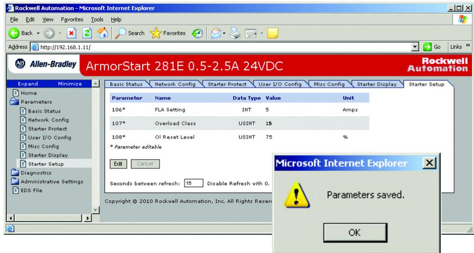
The example screen shows a change of the Overload Class setting to 15. Once all changes are made, select Apply.
