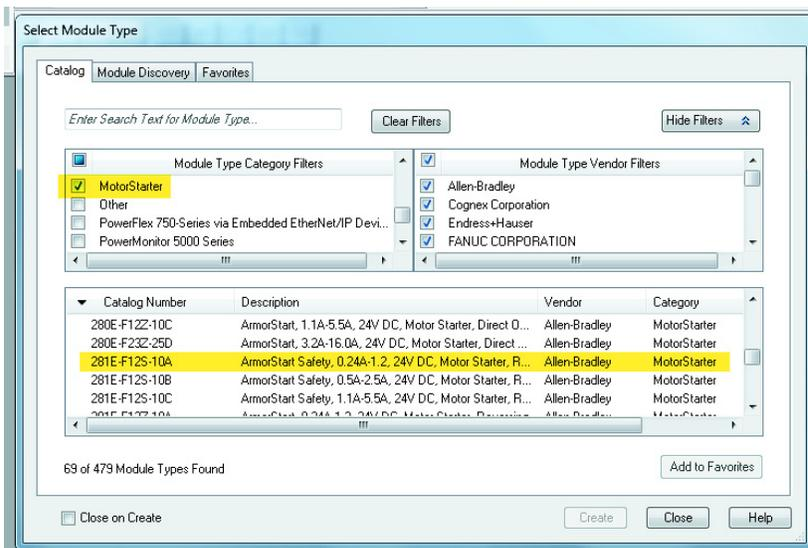
6. The AOP is shown in the next example. Enter a Name for this ArmorStart selection and an Ethernet address. For this example, the Private Network setting is used. This setting must be set to match the IP address switch setting on the ArmorStart selection. Click OK.
