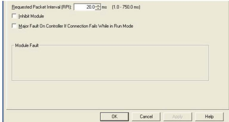
4. From the Requested Packet Interval (RPI) menu, enter the rate at which you want data to be updated over a connection.
