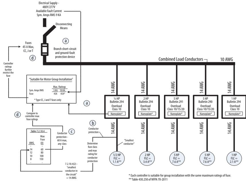
**Figure 94 - ArmorStart LT NFPA 79 Multi-motor Branch Circuit Minimum Conductor Ampacity**
