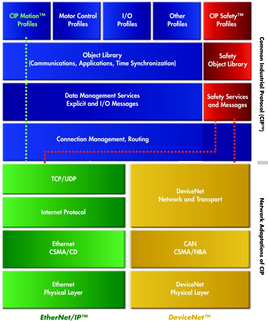
This approach provides real-time technology into the Ethernet domain. With the network extensions of CIP Safety, CIP Sync, and CIP Motion, CIP networks provide for safety communication, time synchronization, and simple-to-high performance motion all over the same EtherNet/IP network.
