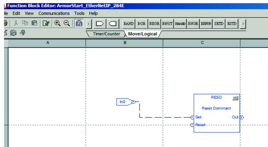
8. From the toolbar, Click the “**Bit Input**” button and select **In 1** from the pull-down menu. This selection is the remote stop button that is based on the example I/O table.
