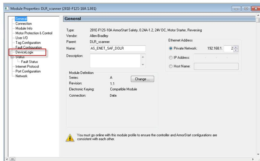
In addition to the actual programming, DeviceLogix can be configured to operate under specific situations. It is important to note that the DeviceLogix program only runs if the logic has been enabled. Configuration can be done within the “Logic Editor.” The operation configuration is accomplished by setting the “Network Override” and “Communication Override” parameters. The following information describes the varying levels of operation:
