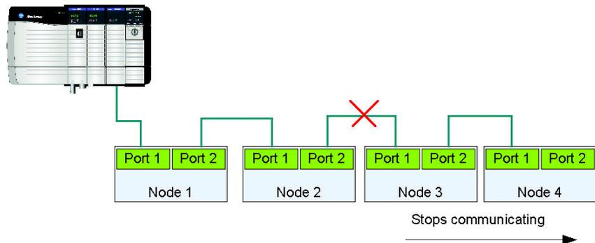
The EtherNet/IP embedded switch technology lets this topology be implemented at the device level. No additional switches are required.
