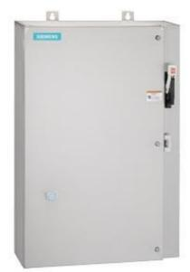
Non-reversing motor starter Size 1 Three phase full voltage Solidstate overload relay OLRelay amp range 10-40a Combination type 30Amp fusible disconnect 30Amp / 250V fuse clip Encl NEMA type 4X 316 S-steel Water/dust tight non-corrosive Extra-wide enclosure
