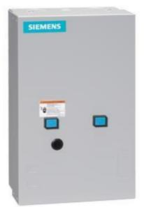
2-speed 3-phase motor starter Size 1 Two separate windings Constant or variable torque Solid-state overload relays Low SPD OLR range 5.5-22A High SPD OLR range 10-40a 110-120/220-240VAC 60HZ coil Enclosure NEMA type 1 Indoor general purpose
