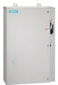
Non-reversing motor starter Size 3 1/2 Three phase full voltage Solid-state overload relay OLRelay amp range 50-200A 550/575-600 50/60HZ coil Combination type 125Amp circuit breaker Encl NEMA type 4X 304 S-steel Water/dust tight noncorrosive Standard width enclosure
