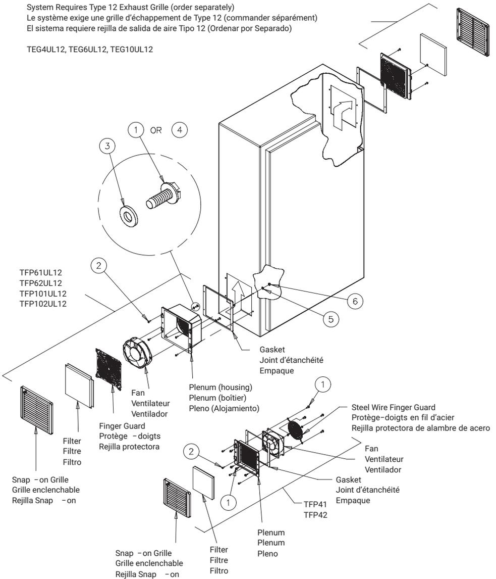
NOTE: To maintain UL type 12 rating, the airflow must be in the direction shown.
