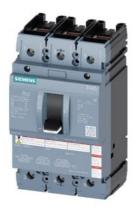
molded case switch 3VA5 UL frame 250 max. sh-circ breaking capacity 100kA @ 480 V 3-pole, line protection MCS110, In=150A without overload protection self-protection li=16 x In cable connection on both sides
