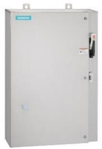
Non-reversing motor starter Size 0 Three phase full voltage Solidstate overload relay OLRelay amp range 5.5-22A 110VAC 50HZ / 120VAC 60HZ coil Combination type 30Amp non-fusible disconnect Encl NEMA type 4X 316 S-steel Water/dust tight non-corrosive Extrawide enclosure
