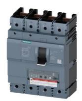
circuit breaker 3VA6 UL frame 400 breaking capacity class L 150kA @ 480V 4-pole, line protection ETU330, LIG, In=250A overload protection Ir=100A...250A short-circuit protection Ii=1.5...12 x In N conductor protection adjustable (OFF, 50%, 100%) ground-fault protection Ig=0.2...1 x In= tg=0.1/0.3s without connection
