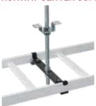
Threaded rod and bracket supports center of ladder rack from ceiling. Kit includes heavy-duty ladder rack cross member, two mounting brackets, two #12-24 screws, 5/8-in. threaded rod, protected sleeve and four 5/8-in. nuts. Use one kit at least every 5 ft. (1.5 m). Made of plated steel.
