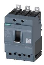
circuit breaker 3VA4 UL frame 125 breaking capacity class H 65kA @ 480 V 3-pole, line protection TM210, FTFM, In=80A overload protection Ir=80A fixed short-circuit protection Ii=10 x In UL489 SB (naval), 50 deg. cel. clamp connection
