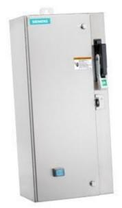
Non-reversing motor starter Size 2 Three phase full voltage Solidstate overload relay OLRelay amp range 13-52a 24Vdc coil Combination type 60Amp non-fused disconnect Encl NEMA type 4X 316 S-steel Water/dust tight non-corrosive Standard width enclosure
