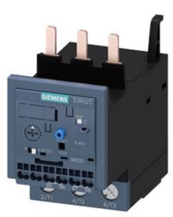
Overload relay 12.5...50 A Electronic For motor protection Size S2, Class 20E Contactor mounting Main circuit: Screw Auxiliary circuit: Spring-type terminal Manual-Automatic-Reset
