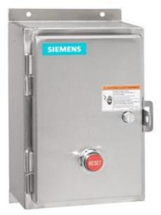
Non-reversing motor starter Size 1 3/4 Three phase full voltage Solid-state overload relay OLRelay amp range 10-40a 24Vdc coil Non-combination type Encl NEMA type 4X 304 S-steel Water/dust tight non-corrosive Standard width enclosure
