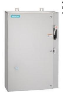
Non-reversing motor starter Size 0 Three phase full voltage Solidstate overload relay OLRelay amp range 0.75-3.4A 24Vdc coil Combination type 30Amp fusible disconnect 30 Amp /600V fuse clip Encl NEMA type 4X 316 S-steel Water/dust tight non-corrosive Extrawide enclosure
