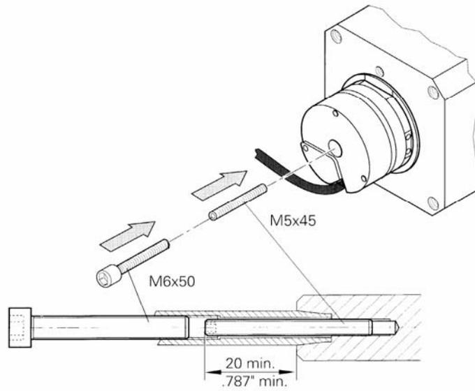
Fig. 7-13 Forcing off an encoder of old design
