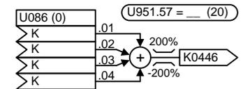
**1 modulo 2^16 adder/subtractor {1 μs}**
