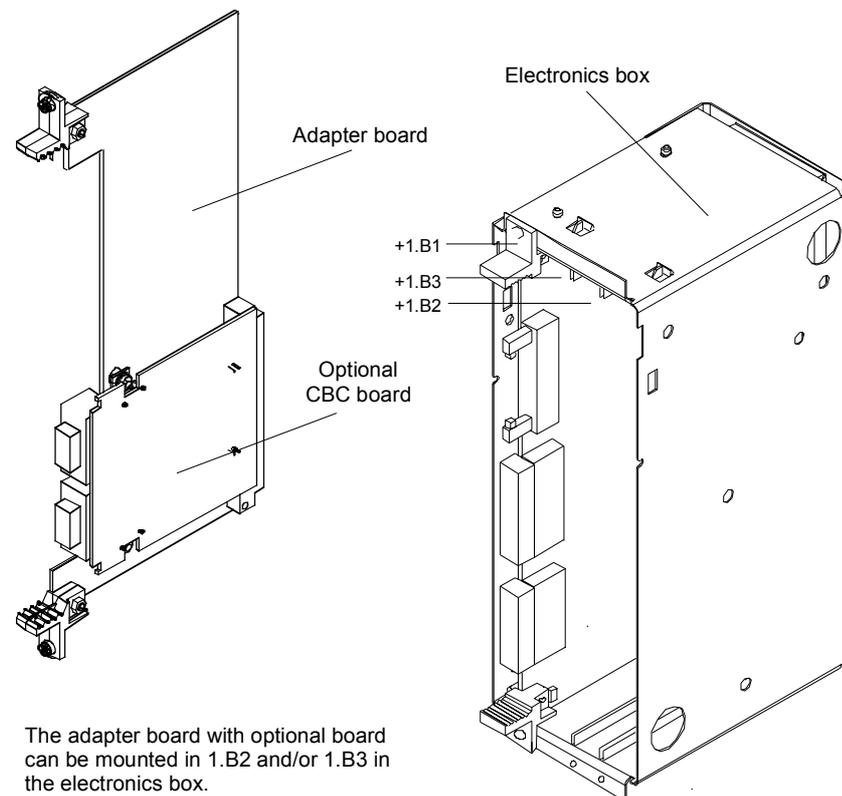
The adapter board with optional board can be mounted in 1.B2 and/or 1.B3 in the electronics box.
