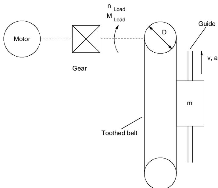
Fig. 11-3 Lifting drive
