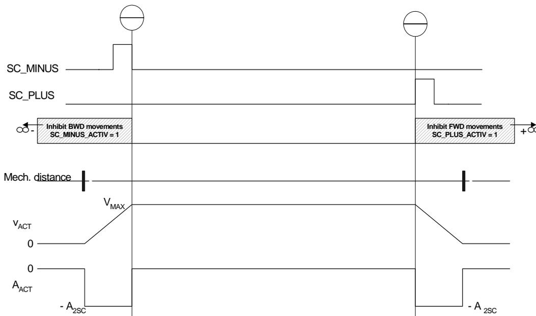
Only movements that lead out of the range of the STOP cams are permissible.
