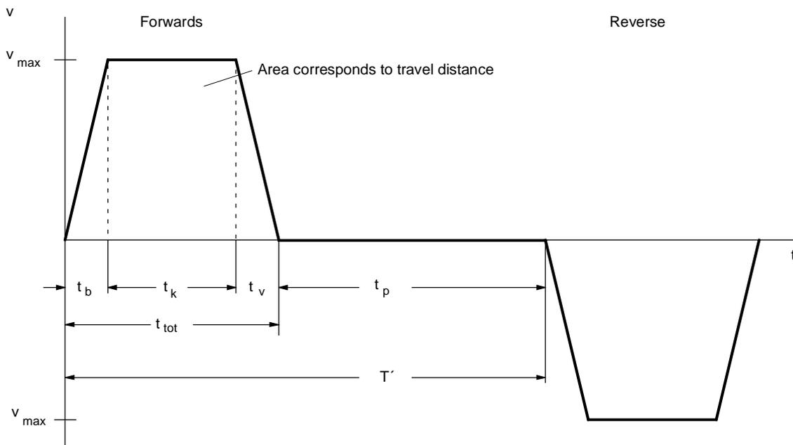
Fig. 11-13 Travel curve for forwards and reverse travel
