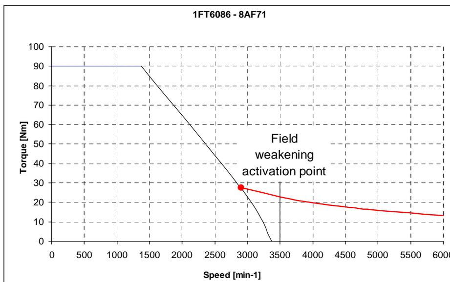
e.g. 1FT6086-8AF71, 27.5 Nm at 2900 rev/min, 13.3 Nm at 6000 rev/min,  $U_{(no\ load\ 2900\ to\ 6000)} = 296\ V$ ,  $I_k(P105) = 37\ A$
