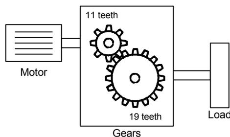
In the example, the motor makes 19 revolutions for 11 revolutions of the load. The value 11 must be entered in U810.01, and the value 19 in U810.02.
