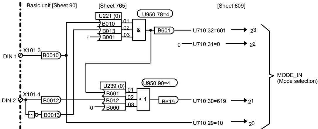
Fig. 9-48 Application example 2: circuit for generating the modes
