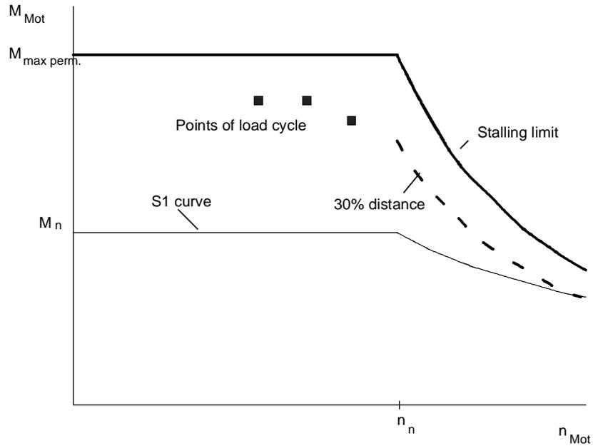
Fig. 11-8 Limit curves for 1PA6 motors (induction servomotors)
