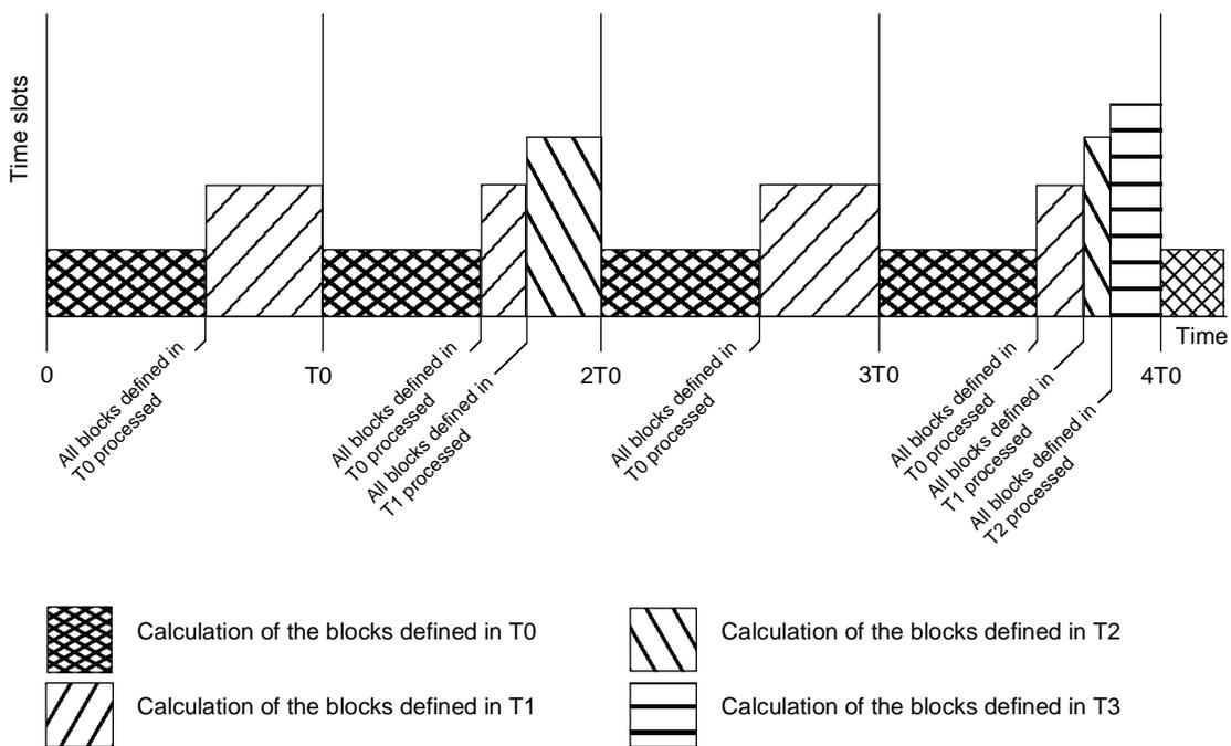
Fig. 7-1 Processing sequence of the time slots
