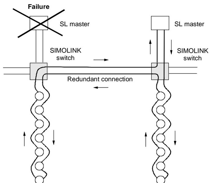
Fig. 8.3-1 Example of an application for the SIMOLINK switch
