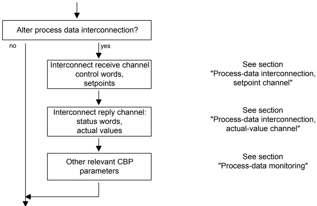
Fig. 8.2-20 Procedure for changing process data
