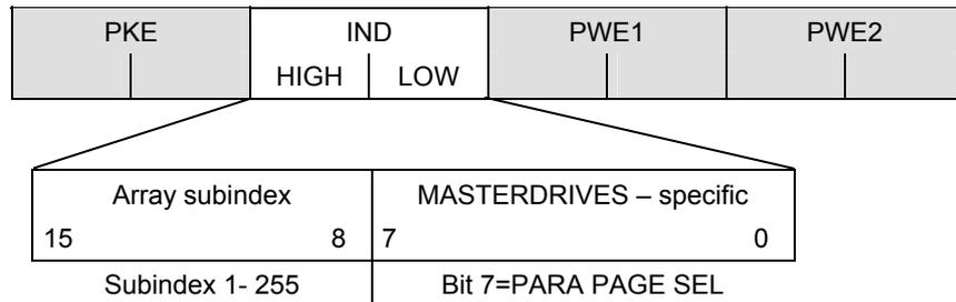
The array subindex is an 8-bit value and, with acyclical data transfer (MSAC\_C1), is always transferred in the least significant byte (bits 0 to 7) of the parameter index (IND). The function of parameter-page selection for additional technology parameters or parameters of free components in the MASTERDRIVES is assumed here by the most significant byte (bits 8 to 15) of the parameter index. This structure corresponds to the stipulations of the USS specification.
