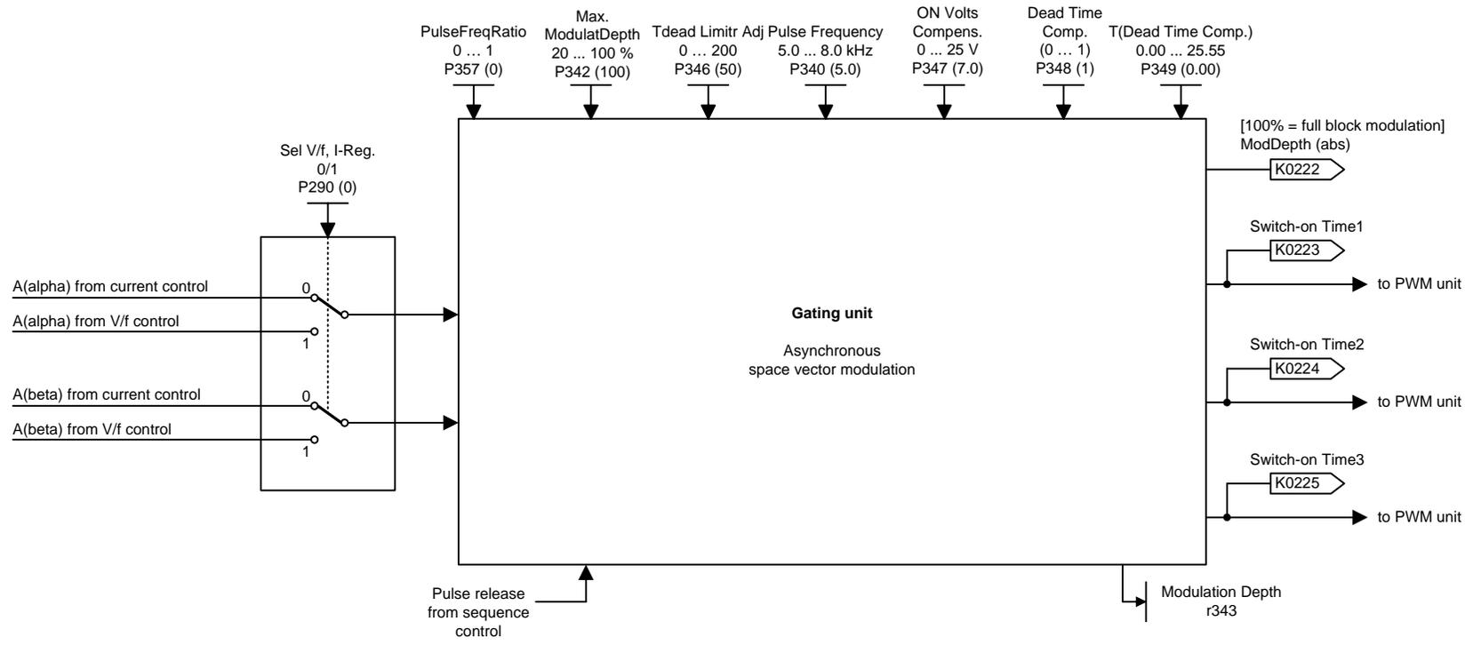
Parameters P348 and P349 are only effective for Compact and chassis units or generally if ASM specialized control is selected (P296 = 3).
