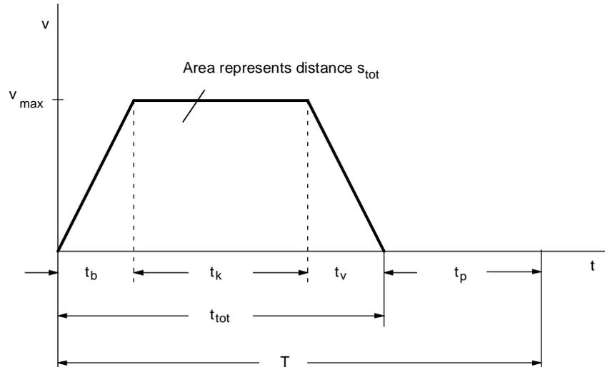
Fig. 11-1 Example of a simple travel curve
