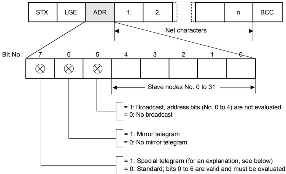
Fig. 8.1-3 Assignment of the address byte (ADR)
