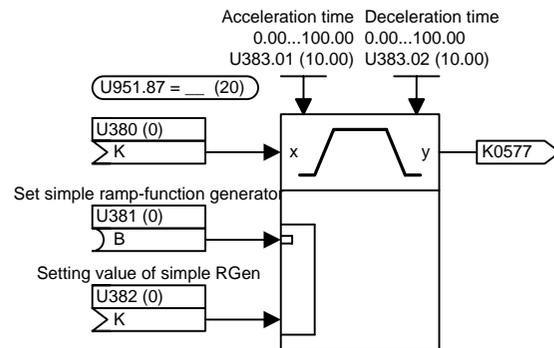
If you wish to use the simple ramp-function generator as a setpoint ramp function generator for the technology controller, the following signal connection can be recommended:
