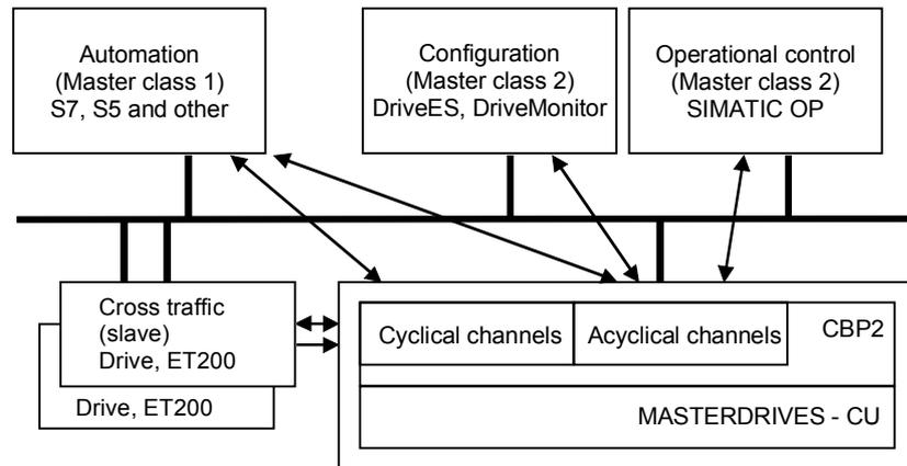
Fig. 8.2-4 Data-traffic channels of the CBP2
