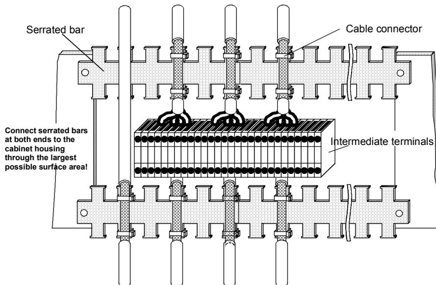
Fig. 3-13 Connecting signal cable shields in the cabinet
