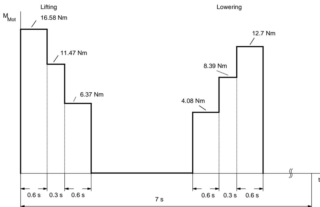
Fig. 11-20 Torque characteristic for lifting and lowering
