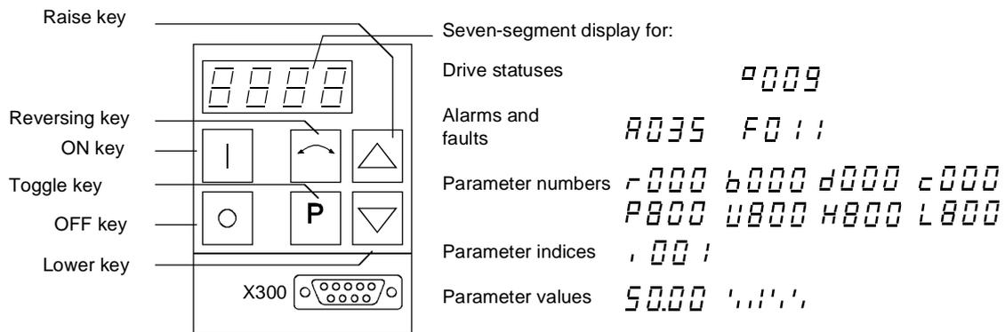
Fig. 5-3 PMU parameterizing unit
