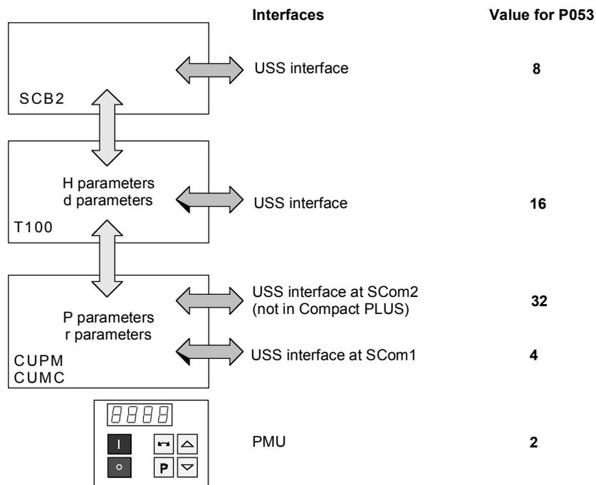
Fig. 8.1-16 Parameterizing enable for the USS interfaces
