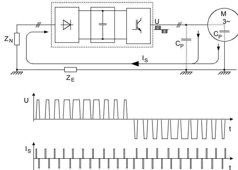
Fig. 3-2 Block diagram showing output voltage  $V$  and fault current  $I_S$
