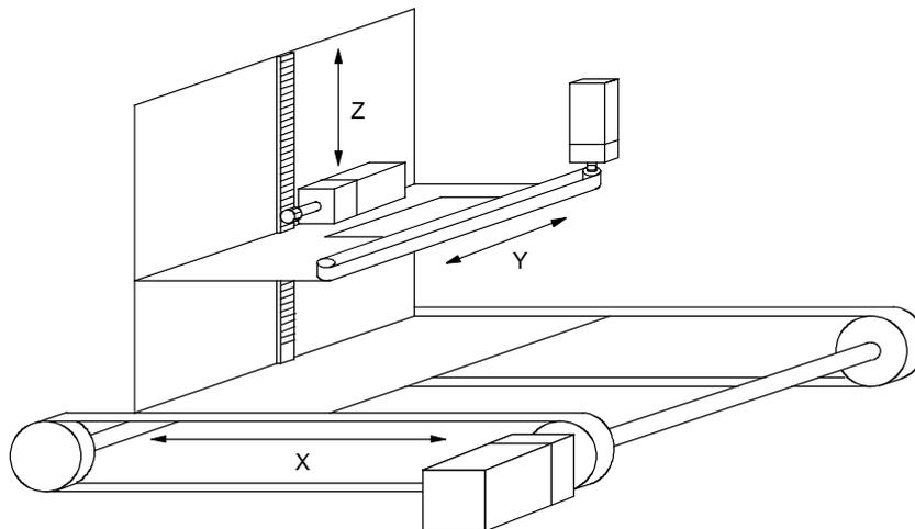
Fig. 11-12 Line drawing of a three-axis conveyor vehicle
