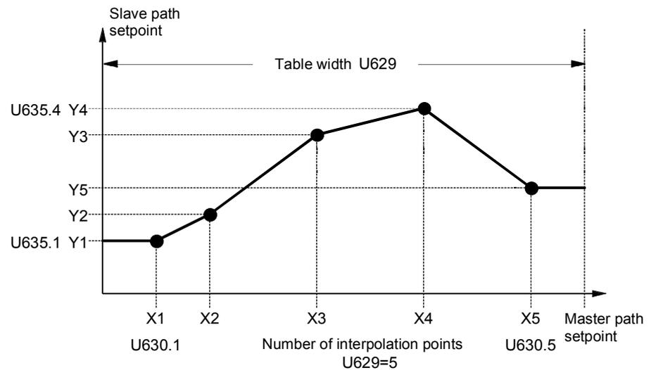
Fig. 9-41 Example of a cam with 5 interpolation points
