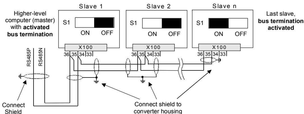
Fig. 8.1-14 Connection of the 2-wire bus cable at terminal strip X100 (Compact PLUS)
