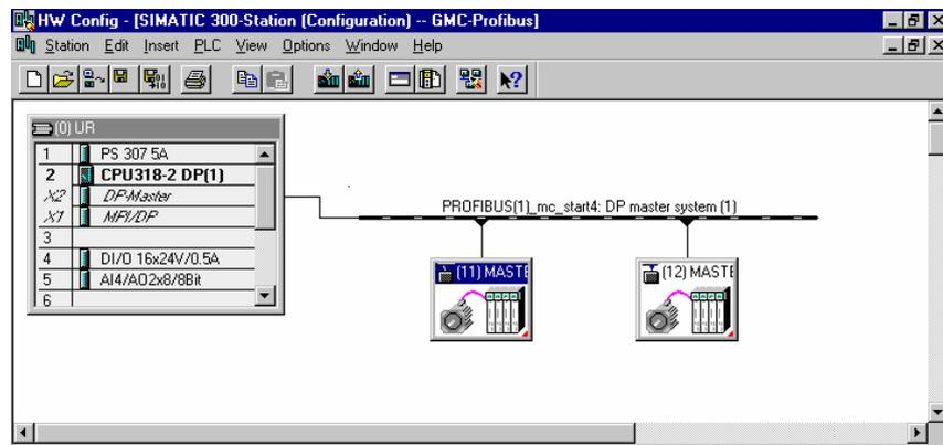
Fig. 9-50 Hardware configuration
