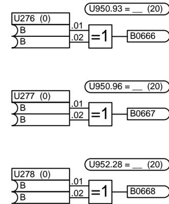
5 digital signal switches {1 μs}
