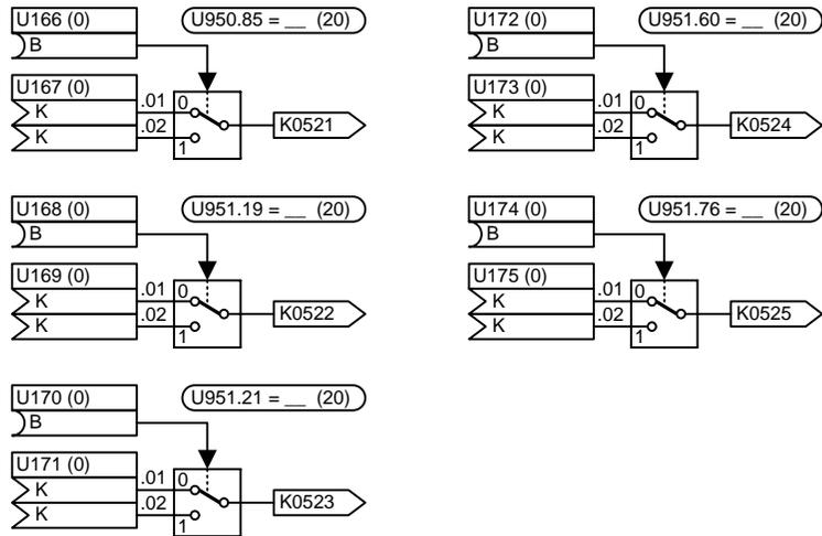
4 Analog signal multiplexer with 8 channels (2-word) {3  $\mu$ s}
