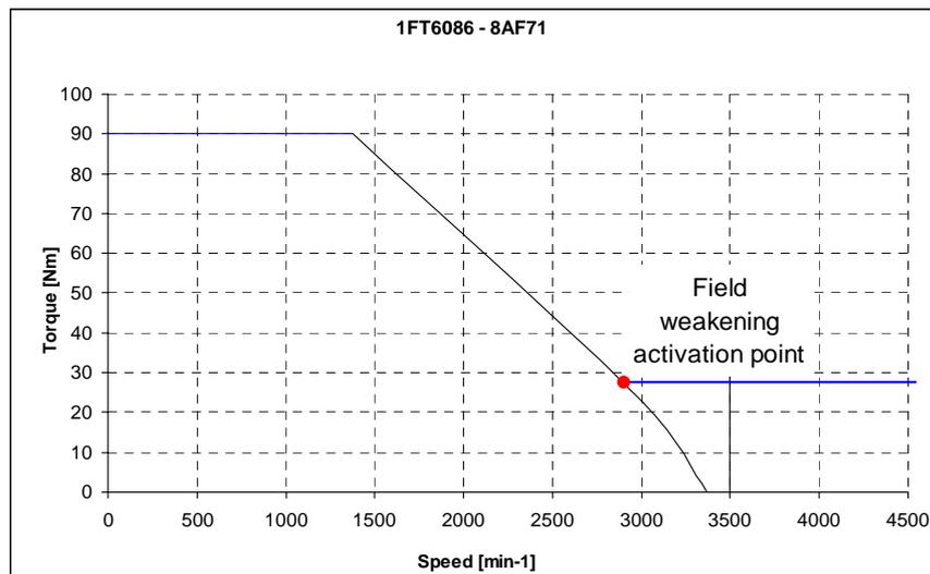
e.g. 1FT6086-8AF71, 27.5 Nm at 2900 rev/min to 4500 rev/min,
