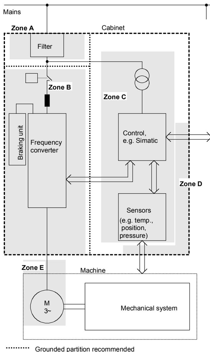
Fig. 3-8 Sub-dividing a drive system into zones
