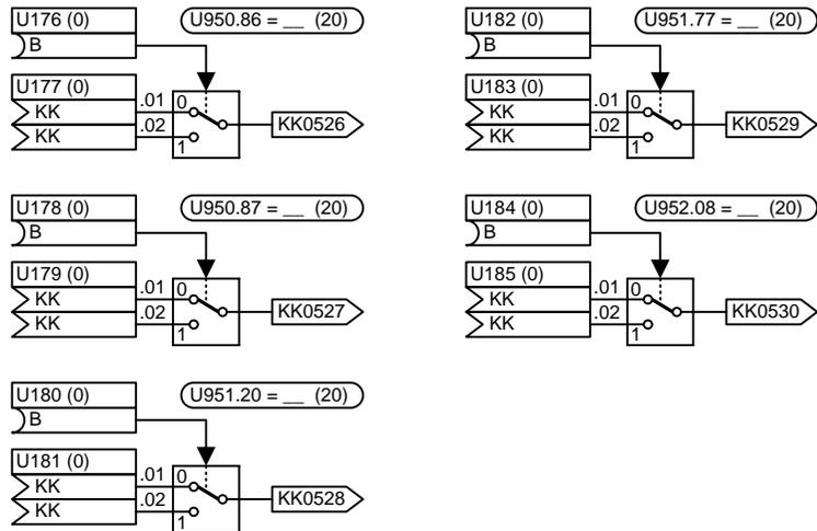
1 Analog signal demultiplexer with 8 channels (2-word) {4  $\mu$ s}
