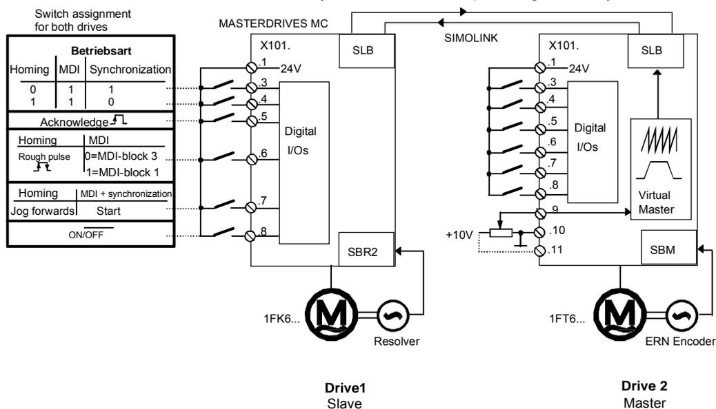
Fig. 9-46 Application example 2: hardware configuration and wiring
