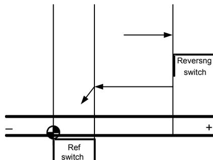
The reversing switch is always active in homing mode. A digital output (MD45 = 8) can be used for connecting the reversing switch.
