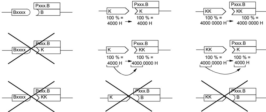
Fig. 4-9 Possible and impossible BICO connections
