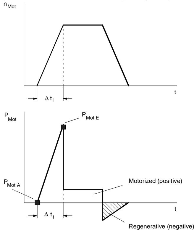
Fig. 11-11 Example of motor speed and motor output in a time segment  $\Delta t_i$
