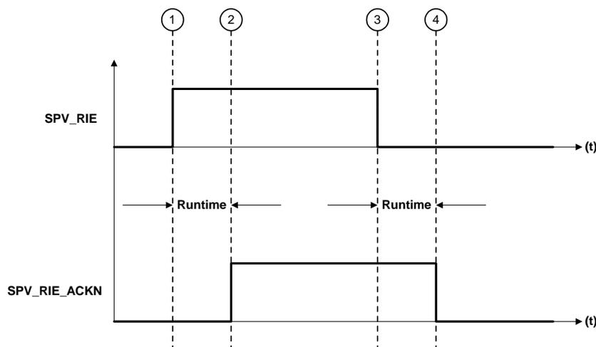
Fig. 7-4 Signal sequence of acknowledgement controlled setpoint transfer
