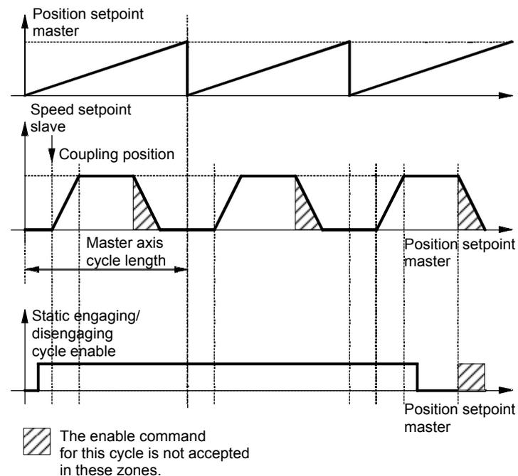
Fig. 9-35 Example: engaging cycle for rotary axis
