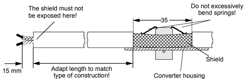
Fig. 8.4-11 Removing insulation from the cable when shield clamps are used
