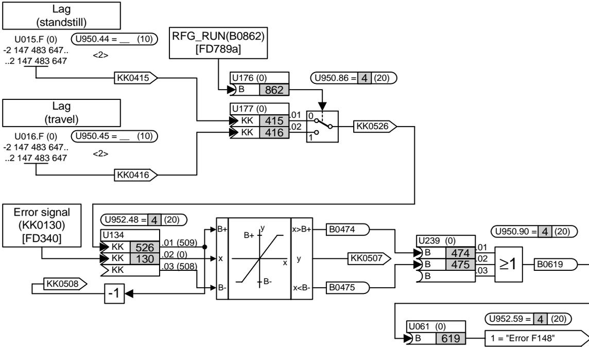
Fig. 7-12 Implement lag monitoring using free blocks
