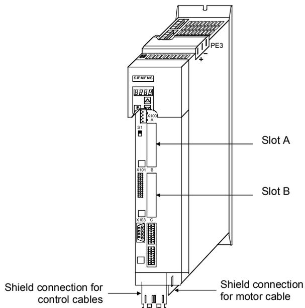
Fig. 8.2-17 Position of the shield connecting points
