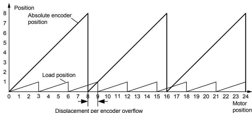
In this case, a load-side offset of  $1/3$  of a load revolution occurs on each encoder overflow, after three encoder overflows the motor and load zero position coincide again. The load position can no longer be reproduced with certainty after an encoder overflow.
