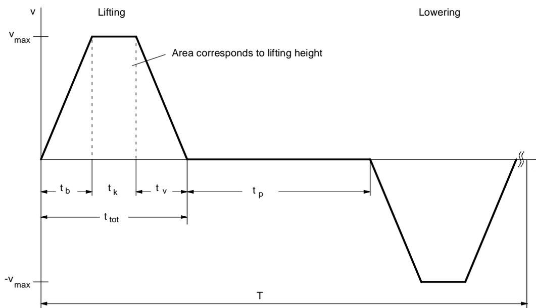
Fig. 11-18 Travel curve for lifting and lowering
