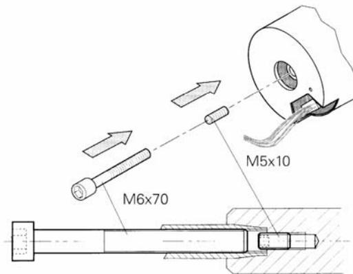
Fig. 7-14 Forcing off an encoder of new design
