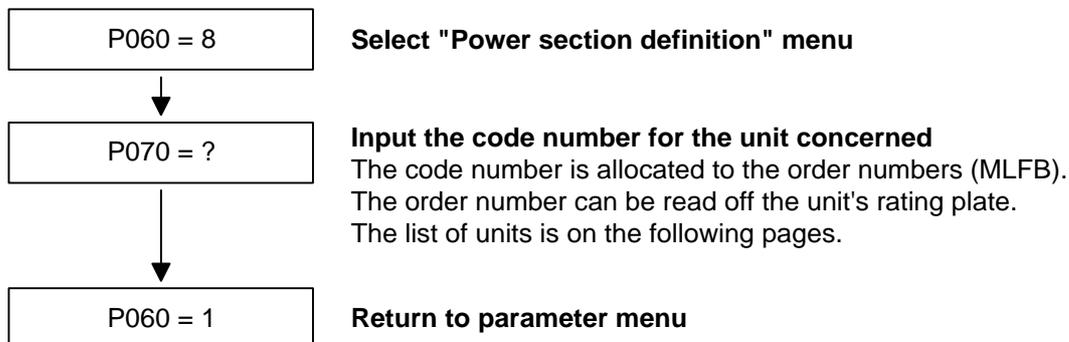
Fig. 6-3 Sequence for performing the power section definition
