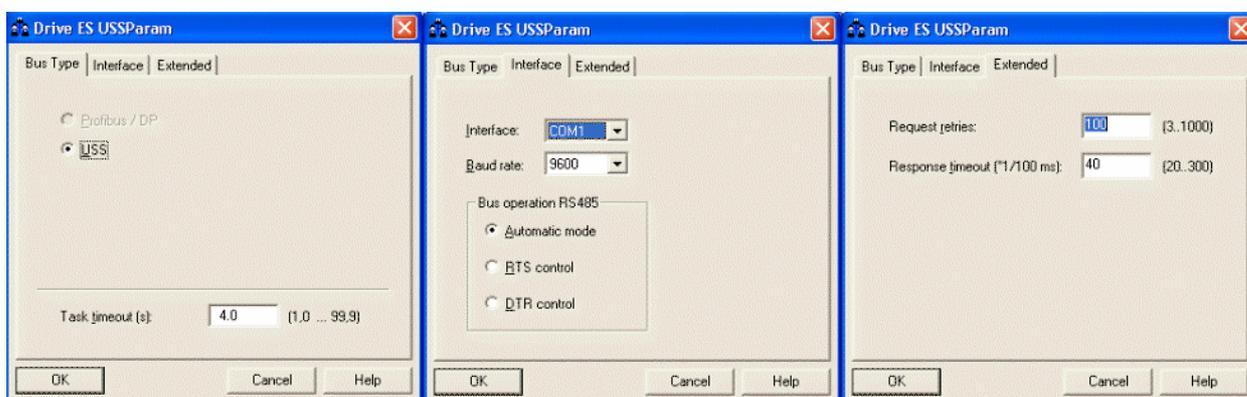
Fig. 5-9 Interface configuration
