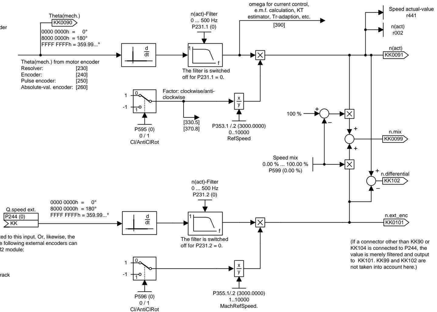
The KK90 can be connected to this input. Or, likewise, the KK104 provided one of the following external encoders can be evaluated with an SBM2 module:
