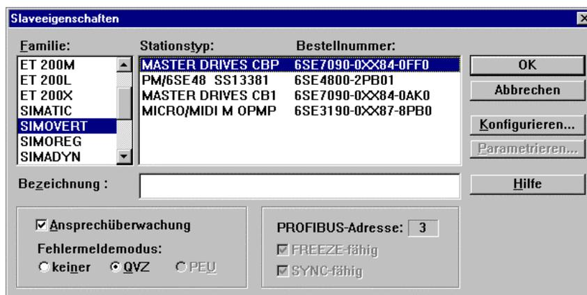
The required type of PPO is selected with this planning tool from a selection table called "Required configuration". This table appears automatically when the menu item "Configure" is selected.
