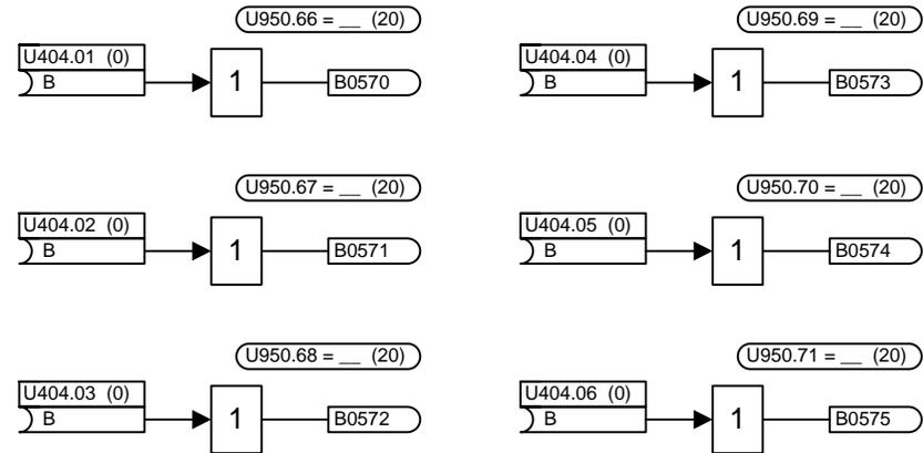
The block does not have any logic function. It only transfers a digital signal consistently from a faster sampling time to a slower one. The block ensures that the signal has the same value in the slow sampling time for all "consumers" (signal sinks).
