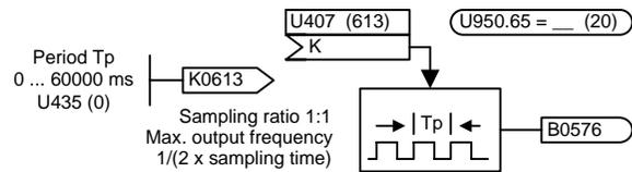
Note: The implemented period  $T_p$  is always an integral multiple of (2 x sampling time).
