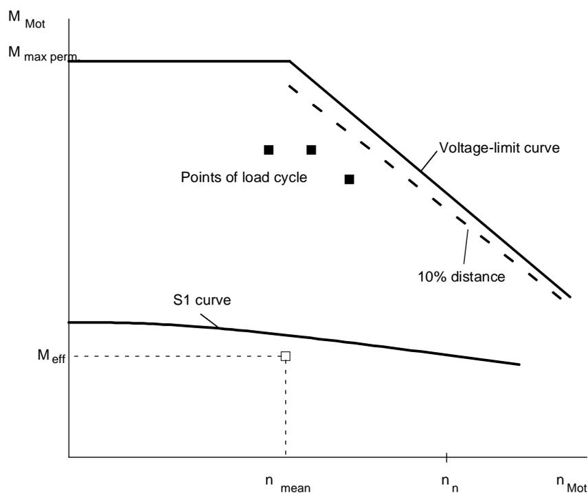
Fig. 11-7 Limit curves for 1FK6/1FT6 motors (synchronous servomotors)
