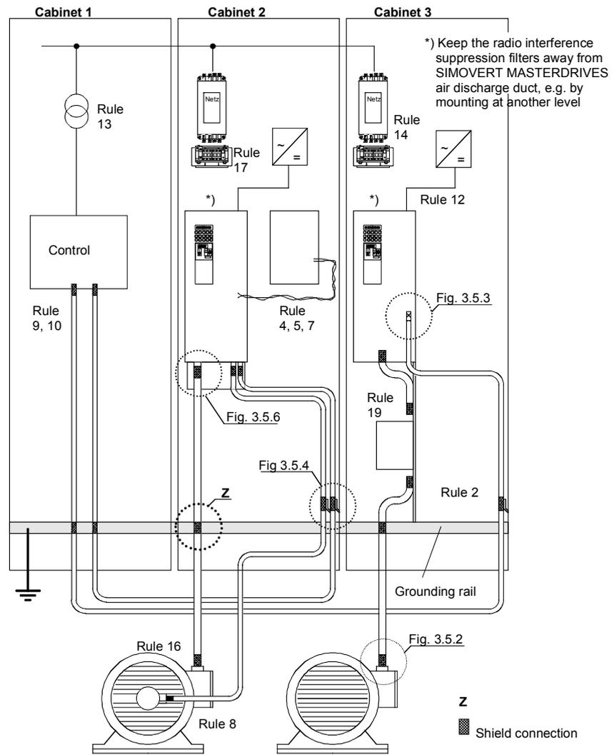
Fig. 3-9 Examples for applying the basic EMC rules
