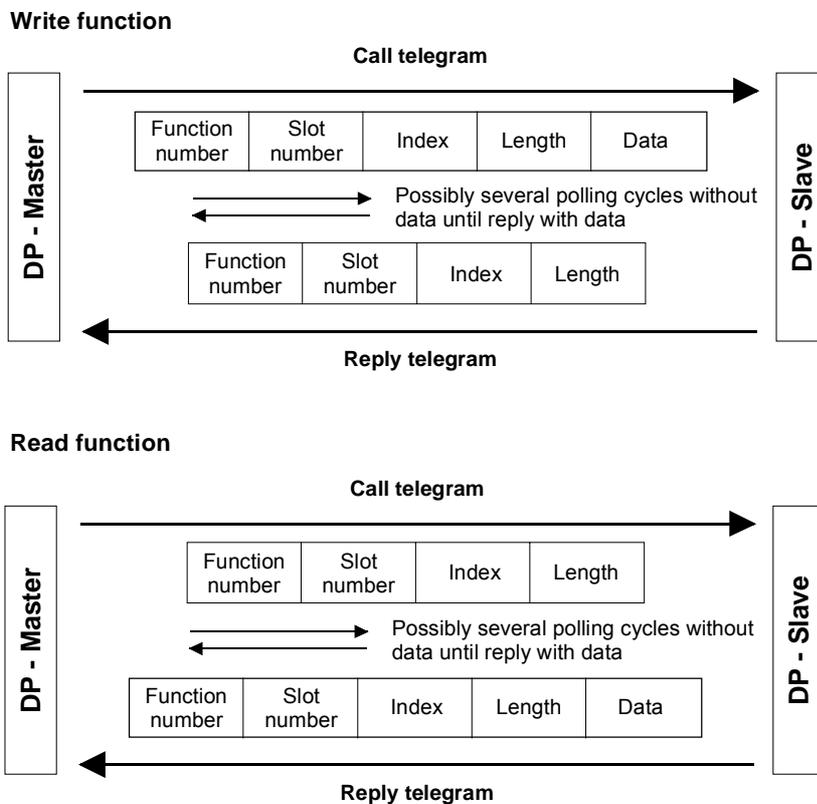
Fig. 8.2-5 Sequence of a Read and Write function
