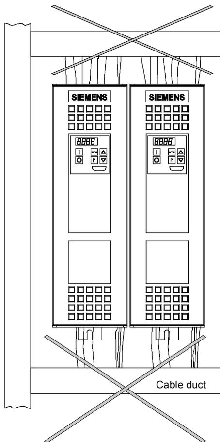
Fig. 3-20 Installation with cable ducts
