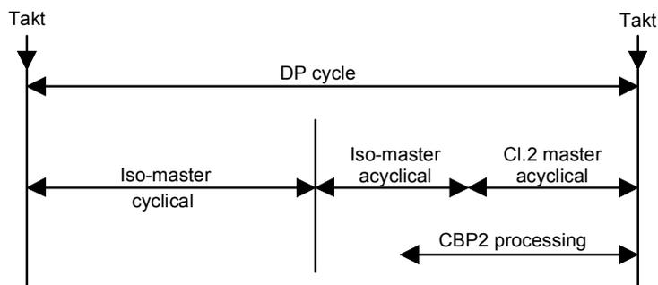
Fig. 8.2-27 Splitting of DP cycle on isochronous PROFIBUS
