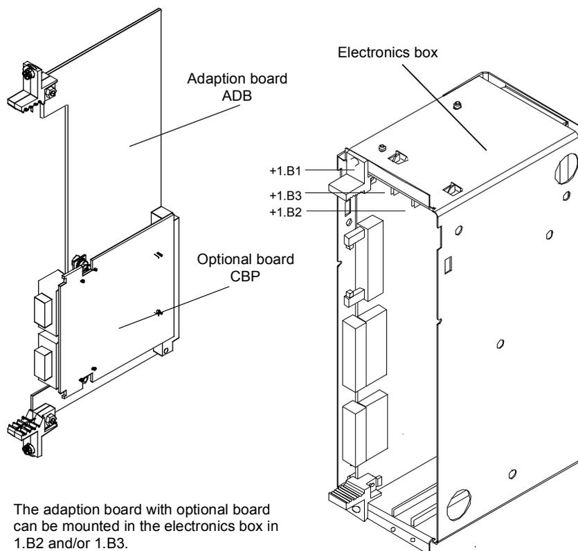
The adaption board with optional board can be mounted in the electronics box in 1.B2 and/or 1.B3.
