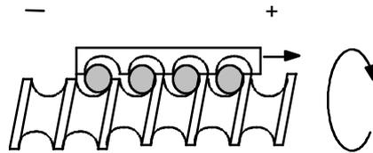
Negative value = negative preferred position → on the first negative movement after switching on the converter, no reverse backlash is taken into account.
