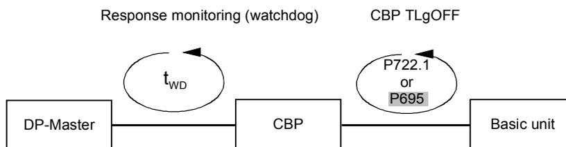
Fig. 8.2-23 Effect of  $t_{WD}$  and P722.1 / P695
