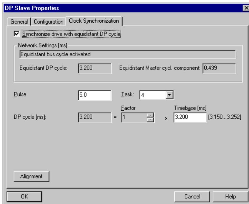
Fig. 9-55 Activation of the equidistance on the converter
