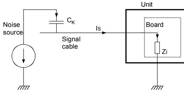
Fig. 3-5 Capacitive coupling for non-shielded signal cables
