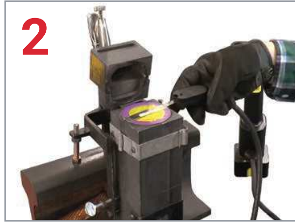
Attach control unit termination clip to ignition strip.
