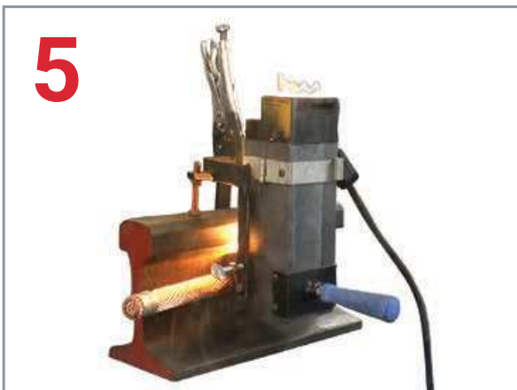
After reaction, open the mold and remove the expended steel cup – no special disposal required.
