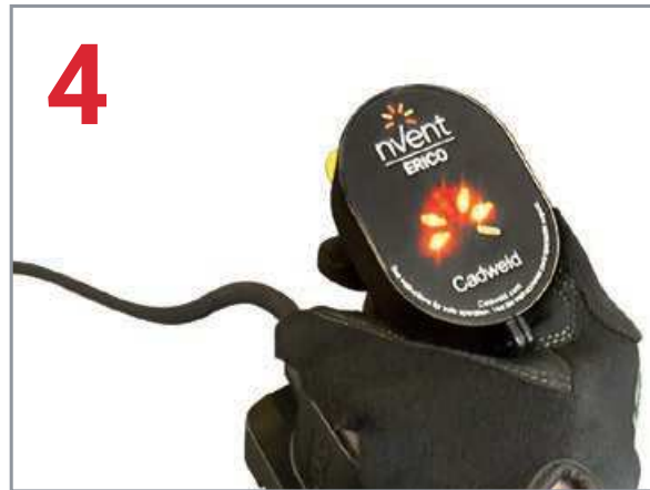
Release the control unit trigger guard, press and hold the switch and wait for the ignition.
