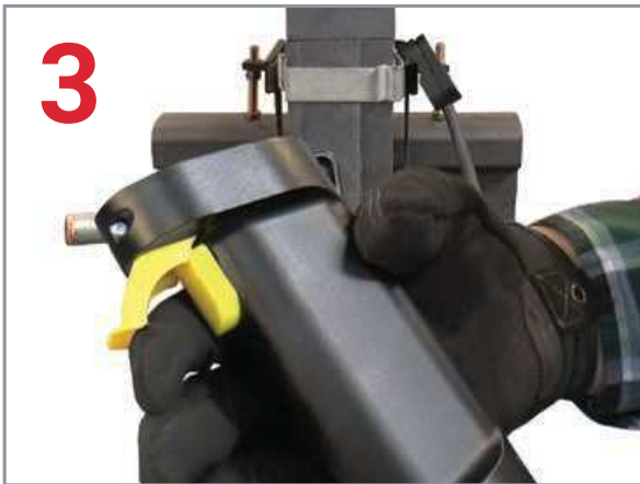
Release the control unit trigger guard, press and hold the switch and wait for the ignition.
