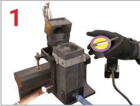
Insert Cadweld Plus cup into mold.
