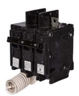
Siemens Low Voltage Molded Case Circuit Breakers General Purpose MCCBs -Type BQ, 2-Pole, 120/240VAC are Circuit Protection Molded Case Circuit Breakers. 2-Pole Common-Trip circuit breaker type BQ. Rated 120/240V (100 A) (AIR 10 kA). Special features: 120VAC Shunt Trip. Note: Load side lugs are included.
