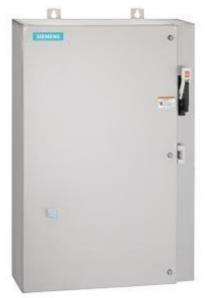
Non-reversing motor starter, Size 4, Three phase full voltage, Solidstate overload relay, OLRelay amp range 50-200A, 110 120/220 240VAC 60HZ coil, Combination type, 200A non-fusible disconnect, Encl NEMA type 4X 304 S-steel Water/dust tight noncorrosive, Standard width enclosure
