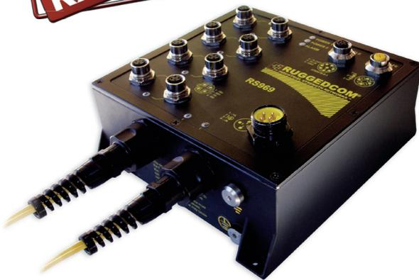
The RuggedSwitch® RS969 is an industrially hardened, fully managed Ethernet switch providing dual fiber optical Gigabit Ethernet ports and eight Fast Ethernet copper ports in an IP66/IP67 rated package for protection against strong jets of water (IP66) or temporary immersion in water (IP67).
