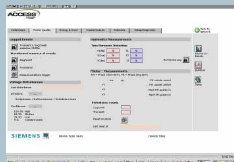
WinPM.Net power quality screen showing data available from the 9610 meter including fault direction detection
