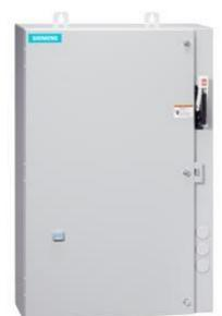
Non-reversing motor starter, Size 0, Three phase full voltage, Solid-state overload relay, OLRelay amp range 0.25-1a, 24VAC 50-60HZ coil, Combination type, 30Amp non-fusible disconnect Enclosure NEMA type 4/12, Water/dust tight for outdoors, Extra-wide enclosure
