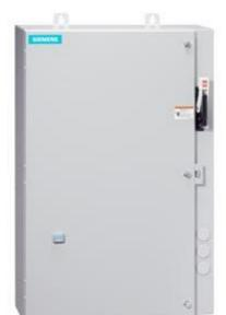
Reversing motor starter Size 2 1/2 Three phase full voltage Solidstate overload OLRelay amp range 25-100A 110VAC 50HZ / 120VAC 60HZ coil Combination type 100A disconnect switch Enclosure NEMA type 4/12 Water/dust tight weather proof
